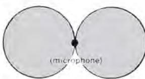
Pick up sound from front and back while suppressing sound from sides, top and bottom.
