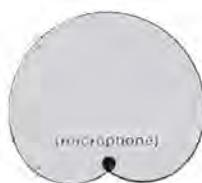
These microphones pick up sound mainly from the front, while suppressing sound and noise coming from the back. The most generally useful unidirectional pickup pattern is the CARDIOID (meaning "heart-shaped"). This pattern will suppress rear sounds at least 70% while picking up front sound over a broad area. Sounds 120° to 180° off-axis are almost entirely suppressed.
