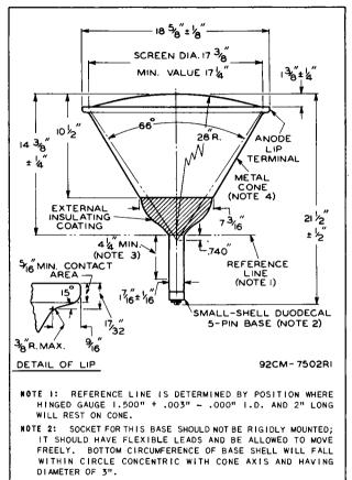
NOTE 3: LOCATION OF DEFLECTING YOKE AND FOCUSING COIL MUST BE WITHIN THIS SPACE.
