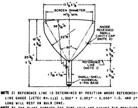
**NOTE 2:** THE PLANE THROUGH THE TUBE AXIS AND VACANT PIN POSITION NO.3 MAY VARY FROM THE PLANE THROUGH THE TUBE AXIS AND ANODE TERMINAL BY AN ANGULAR TOLERANCE (MEASUREO ABOUT THE TUBE AXIS) OF ± 10°. ANODE TERMINAL IS ON SAME SIDE AS VACANT PIN POSITION NO.3.
