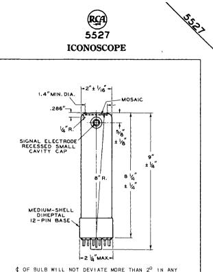
${\bf C}$  of Bulb will not deviate more than  $2^{\rm O}$  in any direction from the perpendicular erected at the center of bottom of the base.
