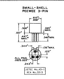
Base-pin positions are held to tolerances such that entire length of pins will enter flat-plate gauge (JETEC No.GA3-1) having thickness of 1/4" and three holes with diameters of 0.1030"- 0.1035" so located on a 0.3440"  $\pm$  0.0005" diameter circle that the distance along the chord between two adjacent hole centers is 0.2340"  $\pm$  0.0005" and the distance along the chord between the remaining pin and the two adjacent pins is 0.3175"  $\pm$  0.0005".
