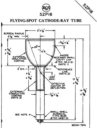
**NOTE I:** THE PLANE THROUGH THE TUBE AXIS AND VACANT PIN POSITION NO.3 MAY VARY FROM THE PLANE THROUGH THE TUBE AXIS AND ANODE TERMINAL BY AN ANGULAR TOLERANCE (MEASURED ABOUT THE TUBE AXIS) OF  $\pm 10^{\circ}$ . ANODE TERMINAL IS ON SAME SIDE AS VACANT PIN POSITION No.3.
