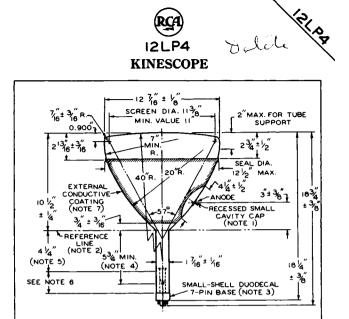
NOTE I: THE PLANE THROUGH THE TUBE AXIS AND VACANT PIN POSITION NO.3 MAY VARY FROM THE PLANE THROUGH THE TUBE AXIS AND ANODE TERMINAL BY AN ANGULAR TOLERANCE (MEASURED ABOUT THE TUBE AXIS) OF  $10^{\circ}$ . ANODE TERMINAL IS ON SAME SIDE AS VACANT PIN POSITION NO.3.
