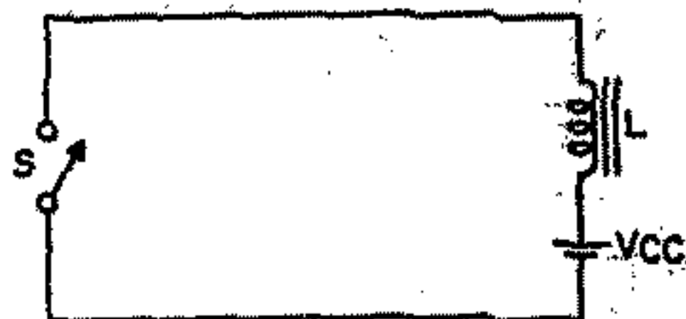
Fig. 85—Simplest form of deflection circuit.
