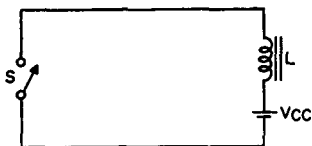
Fig. 85—Simplest form of deflection circuit.
