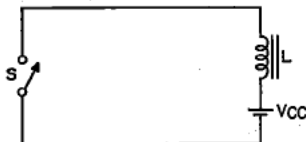
Fig. 85—Simplest form of deflection circuit.
