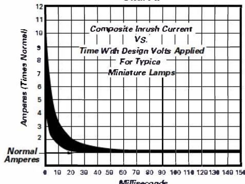
Tungsten filaments are more fragile at temperatures below the 250°C brittle-ductile region. This fragility can be reduced by using a keep-alive voltage or current in the off condition. A general recommendation for keep-alive requirements is 25% of the design voltage or current. This will reduce the inrush current from approximately 12 times to 4 times, depending upon the lamp type.
