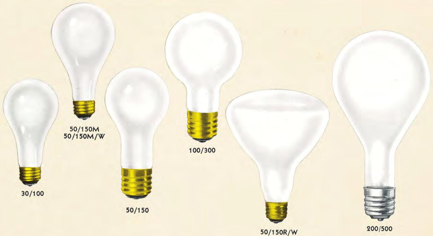
Three-lite lamps with their two filaments provide three levels of lighting. Each filament is of a different wattage and may be lighted individually or in combination with the other.
