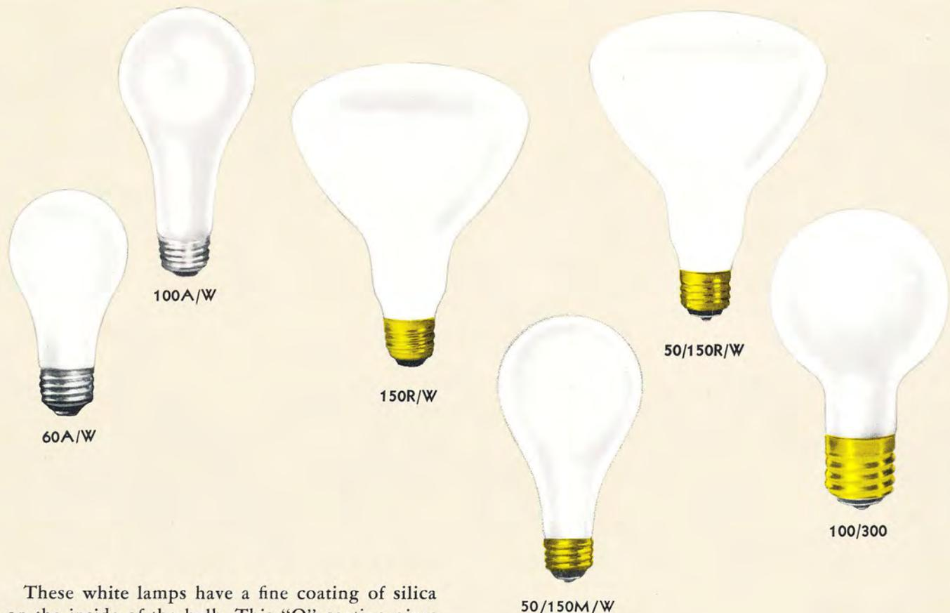
These white lamps have a fine coating of silica on the inside of the bulb. This "Q" coating gives a high degree of diffusion which softens shadows and reduces shiny reflection. The light output of white lamps is approximately the same as that of inside frosted lamps of the same wattage. Since bulb blackening is not apparent through this new diffuse coating the lamps appear clean and white throughout life. The 50/150M/W lamp is for base down burning in floor, table or wall lamps.
