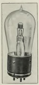
Fig. 130.—General Electric type Receiving Tube. Length: 10 cms.
