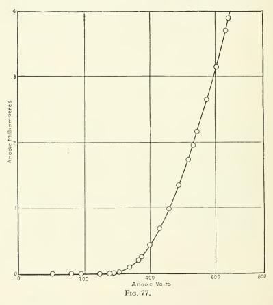
circuit, and the current in the plate circuit observed as a function of the plate voltage  $E_p$ . Since  $r_0$  was zero  $E_p$  was always equal to  $E_b$ , the plate battery voltage. The grid being kept at a constant negative potential  $E_g$  with respect to the filament, current could not be established in the plate circuit until the  $\frac{E_p}{\mu} + \epsilon$  became greater than  $E_g$ . The characteristic obtained is shown in Fig. 77.
