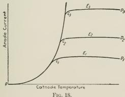
tion current. If the temperature of the cathode be increased to  $T_2$  the curve  $OA_2B_2$  will be obtained. If these values of the saturation current be plotted against the corresponding temperatures of the cathode, the curve shown in Fig. 18 will be obtained,
