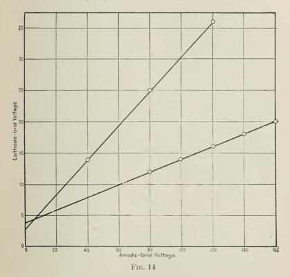
distance d between grid and anode was 6.7 mm., while the upper curve was obtained with d=2.5 mm. If, instead of plotting V as abscissæ, we plot  $\frac{V}{d}$ , the two curves coincide.
