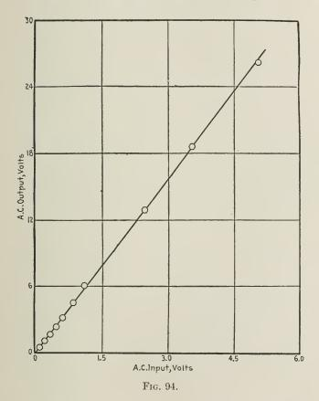
$r_p$  of the tube depends upon the potential difference between filament and plate which, if the voltage of the plate battery remains constant, changes every time  $r_0$  is given a different value. In order to operate the amplifier under the same conditions throughout the experiment, the plate battery voltage should always be adjusted to keep the plate resistance constant.
