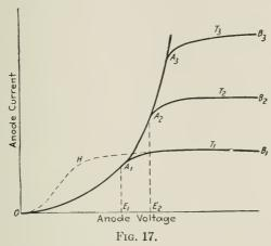
this line is seldom horizontal but usually slopes upward. This part of the curve corresponds to the condition when all the emitted electrons are drawn to the anode as fast as they are emitted from the eathode. The corresponding current is, therefore, the satura-
