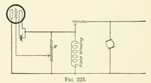
seen that if the current through the resistance R tends to increase, the grid tends to become more negative with respect to the filament, thus increasing the resistance of the tube and decreasing the current through the field winding.
