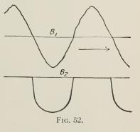
given in Fig. 52 and which was obtained by Dushman. The upper curve gives the voltage across the tube and the lower curve the rectified current.
