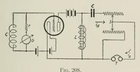
ducing modulated waves. The output of this oscillator system can then be passed through an omnigraph to produce the signals. The R.M.S. of the input can, as before, be measured by means of a resistance r and galvanometer G (Fig. 208).
