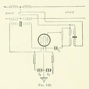
on the grid of the amplifier; these will cause further amplification, the amplification becoming cumulative, thus creating sustained oscillations or "singing."
