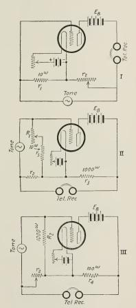
explained above, when  $r_2$  is so adjusted that the tone in the receiver is a minimum, then
