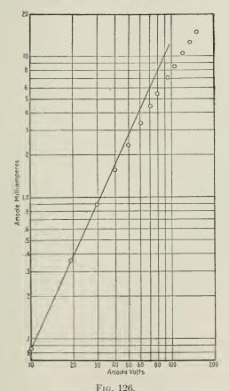
barded by the electrons during the process of evacuation. It contains an oxide-coated platinum filament operating on a normal filament current 1.3 amperes, the voltage being 7 volts. When operated as a telephone repeater the d-c. plate voltage is 160 volts, and the grid is maintained negative with respect to the filament by a battery of 9 volts. The characteristics are shown
