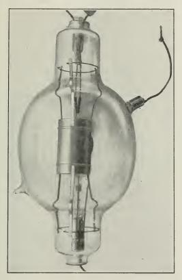
Fig. 135.—British Type Power Tube.
