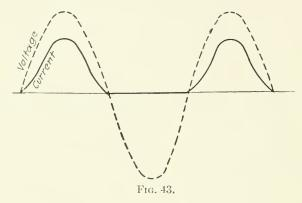
acteristic of the valve. As long as the peak value of the applied simple harmonic voltage is less than  $E_s$  (Fig. 42) when the filament temperature is T the current wave shape takes the form shown by the continuous curves in Fig. 43, the applied voltage being given by the broken curve in arbitrary scale. The departure
