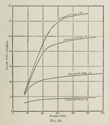
at V. The characteristics of such a valve are shown in Fig. 66. Suppose, now, that the speed of the generator is so low that the
