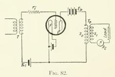
and let a voltage  $e \sin pt$  be impressed between filament and grid. The resistance  $r_t$  may be that of the input transformer coil which is supposed to be wound to work into a practically open circuit. For the present we shall suppose that the external impedance  $Z_0$  in the output is negligibly small compared with the plate-resistance of the tube, so that the characteristic of the circuit is practically the same as that of the tube.
