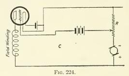
winding are in series. By this means, any tendency for the voltage to increase is counteracted. The same thing, of course, holds when the voltage tends to drop.
