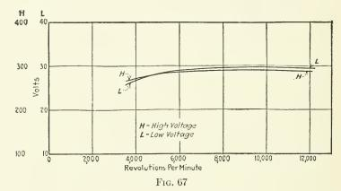
fold increase in the thermionic current. This causes a decrease in the field flux of the generator, thus restricting the increase in the output voltage.
