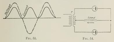
table on p. 77 it is seen that if the filament is of tungsten and is operated at a temperature a little under 2500° K, the thermionic efficiency is 10 m.a. per watt. Since the necessary saturation current  $I_1$  is 300 m.a. the power necessary for heating the filament of the valve under consideration is 30 watts. The power available in the form of unidirectional current in the load can be obtained
