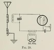
44. The Fleming Valve. This device satisfies condition (3) and has a characteristic such as that shown in Fig. 35 (b). It consists of a filament which can be heated to incandescence and a plate, both placed in a highly evacuated bulb. In 1905 Fleming <sup>1</sup> recognized the use of the rectifying properties of this device for the indication of high frequency oscillations, and used it as a
