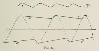
represents the potential of the point D with respect to O, the curves A'A' and B'B' will represent the potentials of A and B respectively with regard to O. The potential difference between A and B is therefore obtained by adding the curves A' and B' and is given by EE. Thus, although the condensers are charged only in alternate
