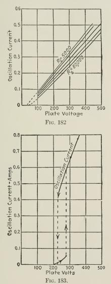
If the plate voltage be further increased, the oscillation current increases almost linearly as indicated in Fig. 183. But if the plate
