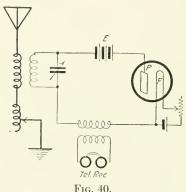
The operation of the device when used this way can be understood from the following: By the insertion of the battery E there is established in the circuit FPE a constant direct current which has a finite value even when no oscillations are impressed from the antenna. The current through the device can therefore be represented by a function of the form
