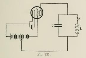
There are various circuits in which the tubes with double grids can be used. In one type of circuit, for example, the grid nearest to the anode is used as an auxiliary anode, while the grid nearest to the cathode operates as a controlling electrode. In this case,
