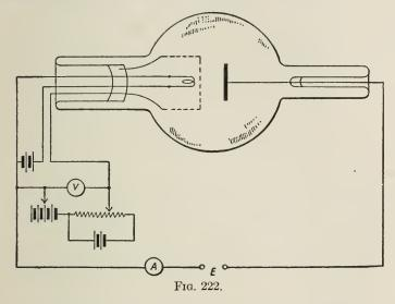
116. The Audion Voltage and Current Regulator. The following circuit arrangements, for which I am indebted to Dr. P. I. Wold, indicate how the tube can be used to control the output of a generator or other source. The generator S supplies power to
