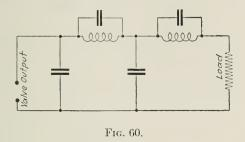
The characteristic of this filter is seen from Fig. 61, where the current attenuation produced by the filter is plotted against the frequency. The capacities and inductances can be so chosen that the fundamental frequency,  $\frac{\omega}{2\pi}$ , is that which gives infinite attenuation. This frequency will therefore not be present in the
