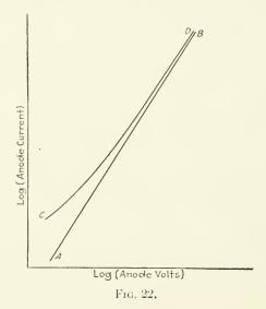
filament which is rendered incandescent by passing a current through it. There is consequently established a voltage drop in the filament which causes a marked deviation from the  $\frac{3}{2}$ -power equation. This deviation is in an opposite sense to that due to the initial velocities.
