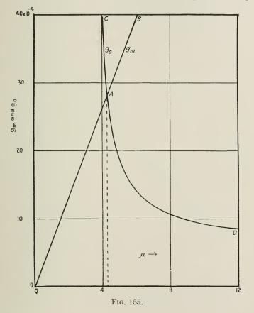
VII, that the mutual conductance is approximately proportional to the plate potential, provided the filament temperature is high enough to insure that by increasing the plate potential we do not enter into the saturation region. We can, therefore, replace  $\frac{\mu}{r_p}$  and  $r_p$  by  $E_p$  and some arbitrary constants. We then obtain
