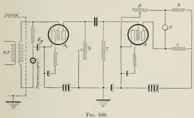
of the tube A, which acts as a detector, so that small potential variations applied to its grid unbalances the bridge.
