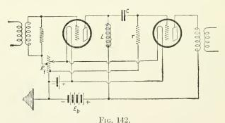
done. Fig. 142 shows a two-stage set in which the first tube is operated as a voltage amplifier. The inductance L has an impedance which is large compared with the plate resistance of the first tube, thus permitting the largest possible voltage amplification. It was shown in Section 62 that if  $L\omega$  is twice as large as the plate
