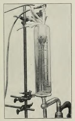
Fig. 138.—Power Tube with Water-cooled Anode.
