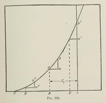
The way in which a wave of the type shown in Fig. 188 is produced by the vacuum tube, becomes apparent when we consider the characteristic. For example, Fig. 189 shows the plate current grid potential characteristic. Suppose a constant potential
