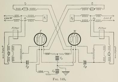
the impedance of the balancing network equal to that of the line to which it is connected, thus making the potentials of the points  $P_1$  and  $P_2$  independent of the currents in the corresponding output coils  $T_2$  and  $T_1$ . This, of course, results in a division of the amplified output power, one-half becoming available and the other half being wasted in the balancing network.
