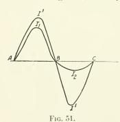
completely block current during the blocking half period. The current wave will then have a shape somewhat like the curve  $I_1I_2$  (Fig. 51). When the valve is short-circuited the current through the external resistance r is given by the curve I'I'. The introduction of the valve not only limits the current in both half periods due to the addition of its resistance in the circuit, but it also
