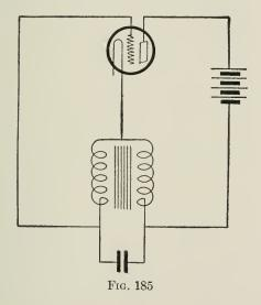
When very low frequencies are desired, it is best to use a Hartley circuit, in which the two coils  $L_1$  and  $L_2$  of Fig. 159 take a form of an iron core transformer such as is shown in Fig. 185. By means of such a circuit it has been possible to obtain frequencies as small as a fraction of a cycle per second.
