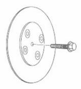
Figure 1-3. Shipping Bolt Removal
