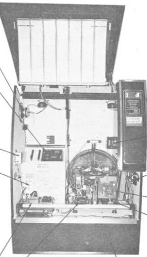
MECHANISM CONTROL UNIT — controls scan, transfer, and toggle shift functions of mechanism.
