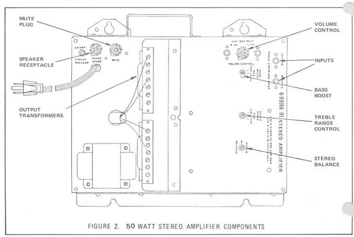
Output Transformers (see Figure 2). The transformers enables the amplifier to operate 70 volt lines for extension speakers. The transformers also provide terminal strips for obtaining several different power levels for both phonograph and extension speakers.
