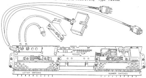
The Tormat Electrical Selector, Type TES108, is part of the Seeburg Tormat Selection System. The principal functions of the selector are to connect a letter and a number circuit of the Tormat Memory Unit of the system into a selection write-in circuit and to complete a circuit that initiates the operational sequence of the system. These are performed when operating a lettered selector key and a numbered key.
