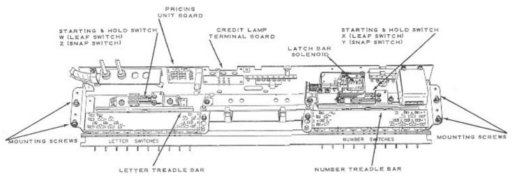
Treadle and Switch Assembly is installed in the electrical selector. The switch of this assembly, \$369, is in the "starting" circuit of the electrical selector. It is normally closed and connecting the starting circuit to the "singles" subtract solenoid in the Dual Pricing Unit. Tabs on the E.P. Treadle may be positioned to actuate the switch when a letter selector button (A to K)
