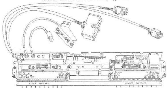
The Tormat Electrical Selector, Type TES106, is part of the Seeburg Tormat Selection System. The principal functions of the Selector are to connect a letter and a number circuit of the Tormat Memory Unit of the System into a selection write-in circuit and to complete a circuit that initiates the operational sequence of the system. These are performed when operating a lettered selector key and a numbered key.
