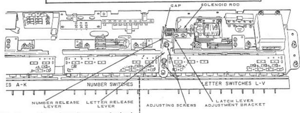
NOTE: When making this adjustment the latch bar solenoid must be in the energized position, all linkage and bars must be free to move without binding and Adjustments No. 1 and No. 2 must be correct.
