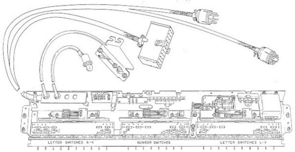
The Tormat Electrical Selector, Type TES165 is part of the Seeburg Tormat Selection System. The principal functions of the Selector is to connect a letter and a number circuit of the Tormat Memory Unit into a selection write-in circuit and to complete a circuit that initiates the operational sequence of the system. These functions are performed when two of the selection switches are operated by pressing a lettered selector key and a numbered key.
