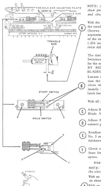
NOTE: All treadle bars should move freely on their pivots to rest against the rubber bumpers and should have a small amount of end play.
