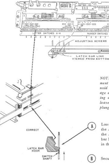
NOTE: Before making this adjustment, Adjustment No. 1 must be correct, the latch bar solenoid must be in the energized position, all linkage and bars must be free to move without binding and there should be a gap between the release lever and the end of the latch bar solenoid plunger rod.
