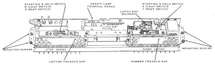
is installed in the Universal Pricing Unit of the phonograph and an E.P. Treadle and Switch Assembly is installed in the Electrical Selector. The switch of this assembly, S369, is in the "starting" circuit of the Electrical Selector. It is normally closed and connecting the starting circuit to the subtract solenoid in the Universal Dual Pricing Unit. Tabs on the E.P. Treadle may be positioned to actuate the switch when a
