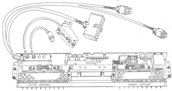
The Tormat Electrical Selector, Type TES107, is part of the Seeburg Tormat Selection System. The principal functions of the selector are to connect a letter and a number circuit of the Tormat Memory Unit of the system into a selection write-in circuit and to complete a circuit that initiates the operational sequence of the system. These are performed when operating a lettered selector key and a numbered key.
