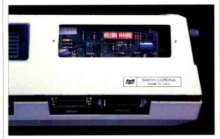
Rear view of printer showing DIP switches.
