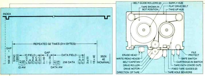
Fig. 1. A disk format of 256 data bytes/sector.
