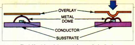
Fig. 4. Metal dome in keypanel gives tactile feedback.
