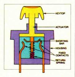
Fig. 3. Mechanical keyswitch.
