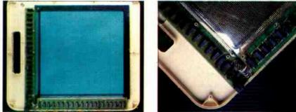
The powerPad uses two plastic grid sheets to form 100 switches per square inch or 14,400 switches per pad.
