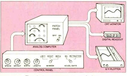
Fig. 1. Analog computer sports car simulator.
