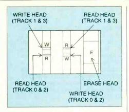
Fig. 3. Read-after-write head.
