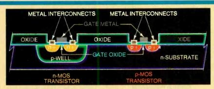
Fig. B. Both p- and n-channel transistors are on one substrate.
