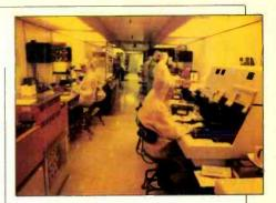
Making CMOS chips at Motorola.
