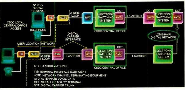
Fig. 1. Block diagram of the circuit switched digital capability
