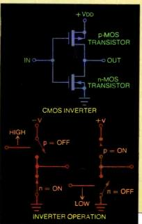
gate was made of metal. The gate formed one plate of a capacitor, whose other plate was the substrate of the device. The two plates were separated by silicon dioxide  $(SiO_2)$ , an insulating material. Because the gate input is a capacitor, the input current is extremely low (for descriptive purposes, it can be assumed to be zero).
