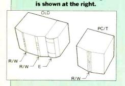
found in the form of the QIC standard. The standard calls for a head with two read gaps, two write gaps and an erase gap—five gaps total. As a result, the head is costly, and maintaining azimuth between the gaps proves difficult. Thus you'll find a simpler head, with a single gap, in Tallgrass's own tape drives. The head actually overwrites a tape, rather than erasing it.
