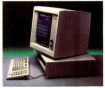
ing unit is an 8-MHz 8086 CPU. Not only does the 8086 have a clock speed faster than the 4.7 MHz of the IBM PC's 8088; it also is a true 16-bit unit. A socket is available for an 8087 math coprocessor.
