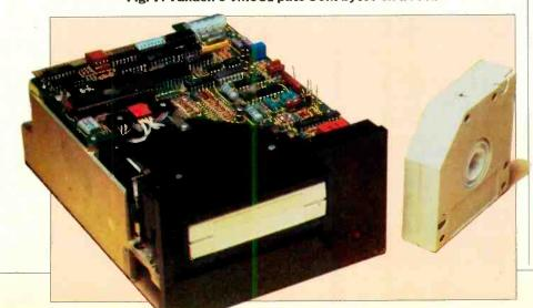
drive, its Series 5000E (Fig. 4), can use either a DC300XL (450') or DC600A (600') cartridge to store from 20 to 60M bytes. The transport senses the type of cartridge you've inserted and automatically makes the necessary adjustments, such as modifying the bias voltage to compensate for different light transmis-
