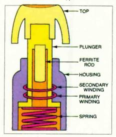
Fig. 2. Ferrite core keyswitch.
