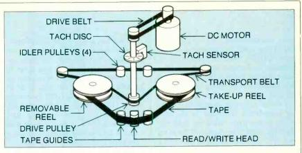
Fig. 6. Interdyne's device uses a self-threading system.
