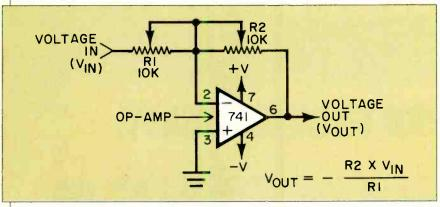
Fig. 4. Basic operational amplifier variable resistor multiplier.
