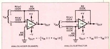
then changing R2's resistance to 50,000 ohms will cause the output voltage to equal the average of the two input voltages.
