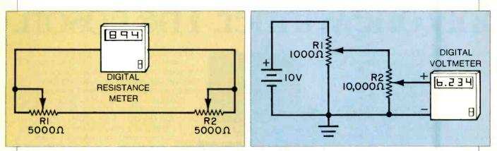
Fig. 2. Variable resistor analog addition circuit.
