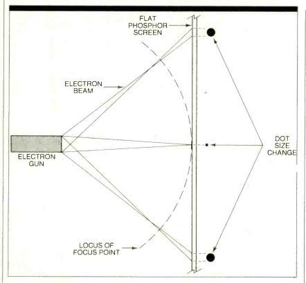
Fig. 5. Electron beam focus changes as screen is swept.
