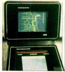
Touch screen controls radio, interior climate, navigation and compass.
