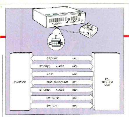
Fig. 5 PCjr joystick connections.
