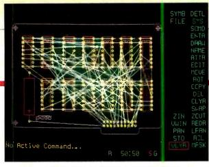
Mouse-driven menu is on the right side of screen. Drawings can be layered to show components.
