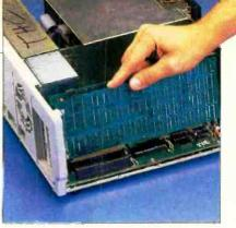
The 1000 can accommodate three IBM-compatible expansion boards.
