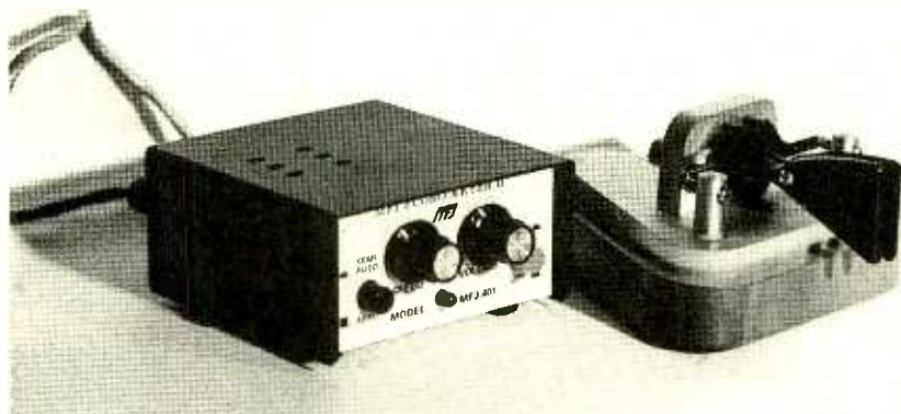
The MFJ-401 Electronic Keyer (from MFJ Enterprises) and a Vibroplex key. The Vibroplex key—essentially a paddle-operated single-pole double-throw switch—is especially designed for use with electronic keyers. The MFJ-401 keyer offers speed control, and the ability to effect a contact closure on dash in order to simulate a bug and to tune-up transmitters.
