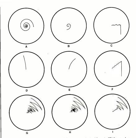
Fig. 6. Oscilloscope displays of some of the different traces obtained from the STAR tester. In trace patterns (A) and (B) are shown good inductors. Trace (C) shows an open winding, or no leakage. Traces (D) and (E) show shorted turns. Trace (F) shows leakage. Traces (G). (H), and (I) show typical yoke-winding patterns.
