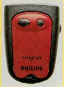
The numeric pager is the smallest and lightest in its class. It stores up to 32 time-stamped messages, with up to 20 messages protected. Messages can be deleted individually, and duplicate messages are automatically eliminated.
