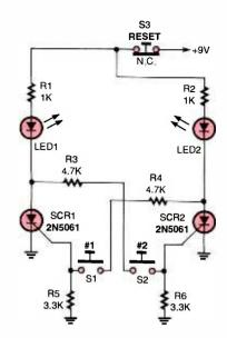
Fig. 4. Who has the fastest reflexes-operator #1 or #2? The first one to press the switch does! This circuit can be used to compare response times or as an indicator in a quiz show gameuse your imagination to think up all the applications!
