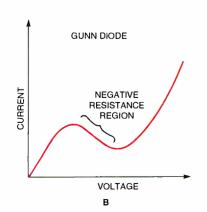
Fig. 3. Graphs showing the current and voltage **62** for normal (A) and Gunn diodes (B).
