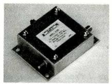
The ICE Model 430B TV highpass filter, shown here, passes signals from 54 to 500 MHz and employs a variety of techniques, including a deep-notch, low-end cutoff attenuation slope below TV frequencies. A similar unit, the Model 436B, eliminates FM broadcast interference. The Model 437B incorporates a notch filter for the two-meter amateur band.
