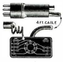
The 666's "probe" (above) had a tube base at one end and a grid cap at the "other." It was connected via cable to the "test block" (below).
