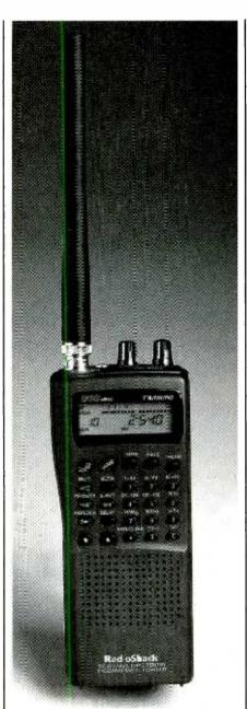
RadioShack's PRO-91 TrunkTracker allows you to monitor conventional VHF/UHF systems as well as most of the popular 800-MHz trunked systems.
