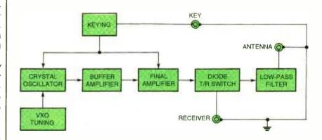
Fig. 1 Block diagram of the ORP-30 transmitter.
