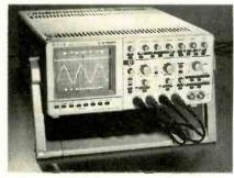
Dual-channel capability includes functioning as a dual-trace scope in the differential mode. The 5034 includes full differential inputs on both channels and external trigger input. The oscilloscope features a digital refresh rate of 0.1 µs to 200s/div, 40-MHz sampling frequency, and sweep speed of 0.2 µs/div in 1-2-5 sequence, 20 positions. DC-coupled frequency response ranges are to 20 MHz (channel 1) and 30 MHz (channel 2). An RS-232 port enables hard-copy and remote programming (SCPI).
