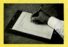
Using a digital pen equipped with an RF transmitter, you take notes on a standard  $8^{1}/_{2^{-}} \times 11$ -inch lined notepad affixed to the *CrossPad's* digital notepad. Meanwhile, signals from the digital pen are stored as digital notes in the pad's memory. The keyword feature allows you to circle a word and search for it later, making it easy to retrieve your notes. Change pages by flipping the page over.
