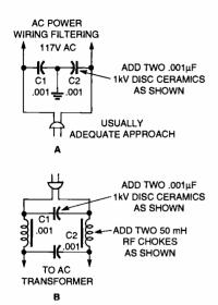
Fig. 2. An AC power-line filter can prevent RF from a nearby transmitter from entering the TV or other device via the power cord. The filter may be purchased or you can build a simple unit yourself. Note that the filter circuits shown here aren't the same as surge suppressors, although both functions may be combined in a unit.
