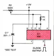
Fig. 6. Here the venerable 555 oscillator/timer IC is used as an astable oscillator. The frequency of oscillation is determined with resistor R1, potentiometer R2, and capacitor C1. The duty cycle is set with R1 and R2.
