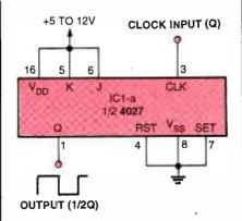
Fig. 4. In this circuit, a single IC, the 4027 dual JK flip-flop, operates in a divide-by-two configuration. The output is one-half of the input clock rate.
