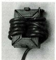
Snap-together toroid chokes can be effective in curing RFI; you can use them on telephone, computer, power, audio, and coax lines. With this core, you don't have to cut the cable-simply wind the wire or line through the core. (Photo courtesy Radio Shack)
