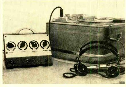
Output of the second recorder feeds into monitor earphones, permitting you to hear previously recorded "tracks" as you add another. Mixer is shown at left.
