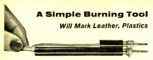
HERE'S a burning tool you can make in half an hour. You can probably find all the materials in your junk box, or at most, they would cost you \$3 to \$4 at any parts store. The transformer is a 6.3-volt filament transformer capable of delivering 3 or more amps. The 100-ohm, 5-watt rheostat is the temperature control. A short length of Nichrome wire makes up the burning tip, which you can attach to the ends of an ordinary pair of test prods.
