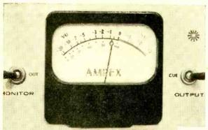
Volume indicators of three different kinds are used on tape recorders. At left is the professional-type VU meter which monitors the level of every sound entering the machine. The "electronic eye" in the tape recorder below serves the same purpose. The machine in the bottom picture has a neon bulb, which flashes overload warnings but cannot indicate intermediate values of signal level.
