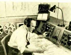
This RFE monitor records the frequency, language, time of day and station of every broadcaster on the short-wave bands. The chart is then used to plot broadcast channels and to locate free channels.
