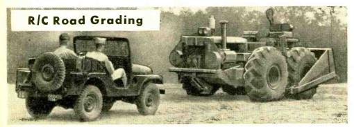
Push-button construction work is on the way. A standard U.S. Army "Tournadozer" equipped with standard military radio equipment (above) can be put through its paces by helicopter or jeep with transmitter and special control box up to a distance of 15 miles. It's under test at Fort Belvoir, Va.
