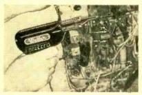
NEW SOLDER FOR CATHODE TUBE BASE PIN. Defectively soldered (or loose) base pin is re-sweated to remove imperfections. New solder is then applied to establish uninter-upted contact. Weller Gun is ideal for this type of repair.
