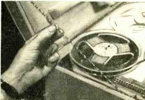
chain from the recorder case up to the lid, and fasten it at both ends with small screw eyes. Leave one screw open so that chain will unhook for cover removal.—*R. A.*
