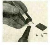
or blow out excess solder. Use a file to cut a groove in the Bakelite portion of the holder just wide and deep enough to fit snugly over the twin-lead you are using. Next, strip the conductors of the twin-lead back  $\frac{5}{8}$ " to  $\frac{3}{4}$ ", clean and pre-tin them. Push them fully home in the crystal holder pins, solder, and reassemble the holder. Any standard crystal socket serves as a female connector on the receiver chassis. —Waldo T. Boyd
