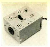
In addition to mounting D1 on heat sink, ventilation holes should be provided to dissipate heat generated in operation.
