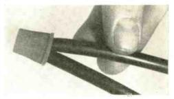
will serve almost as well, if you twist the wires together and trim them fairly short. For a permanent connection, put a little speaker cone cement or other adhesive in the cap before you screw it on.
