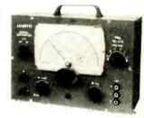
380 mc. Outputs are unmodulated r.f., modulated r.f., and 400 cycles audio. The r.f. output is in excess of 100,000 microvolts. Stability is insured by a circuit which uses a 12BH7 twin-triode cathode follower-buffer and a 6AR5 a.f. oscillator. The a.f. output is 2-3 volts, a.f. input 4 volts across 1 megohm. Price, \$27.95. (*Lafayette Radio Electronics Corp.*, 111 Jericho Turnpike, Syosset, L.I., N.Y.)
