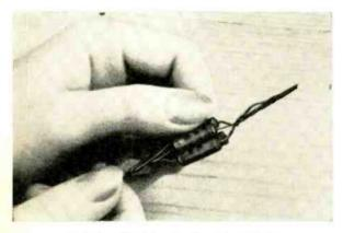
In the politest terms, these four resistors can be called "floor sweepings." Twisting the leads together was done by a technician, eliminating the chance that the resistors would be new stock. "BAD" ASSORTMENT
