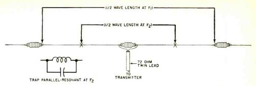
By substituting traps for insulators at "X" points, one dipole will work on two bands.
