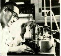
Reversing the usual procedure, power can be fed to a biocell to produce chemical reactions. Above, Dr. Y. H. Inami does so in a NASA study to simulate reactions that occur in biocells.
