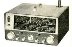
SPECIFICATIONS—IF Frequency: 455 kc. Frequency coverage: 550 kc to 32 mc in 5 bands with calibrated bandsbread scales (oscillator tuning) for 80. 40, 20, 15 and 10 meter amateur bands and 11 meter citizens band. Selecttivity: 3 kc wide at 6 db down. Sensitivity: 10 uv broadcast band, 2 uv short wave bands for 10 db signal-to-noise ratio. Output: 400 milliwaits max. Battery life: up to 400 hours normal intermittent service using 8 standard size "C" cells. Dimensions: 6%"H. x 12"W. x 10"D.
