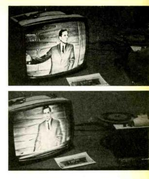
tape home movies. The American model of the machine records up to 44 minutes of sound and video on an 11" reel of ordinary audio tape using two tracks at 22 minutes per track.
