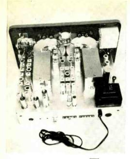
or both), and a four-position selectivity control that permits the receiver bandwidth to be varied from .5 to 3 kc. on either sideband, or from .5 to 6 kc. on both sidebands.
