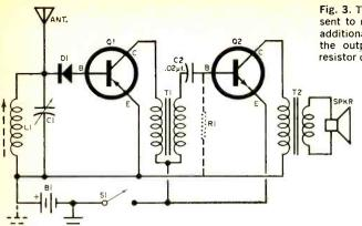
Fig. 3. This receiver circuit was sent to us by Kenneth Baer. If additional bias is necessary for the output stage, a half-watt resistor can be added as shown.
