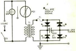
Vertical line between lamp and photocell in schematic diagram represents shutter vane. Circuit is shown with plus side of output grounded, but may be left floating if both output terminals are insulated from box.
