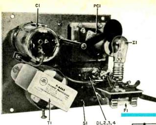
Mount all parts far enough in from panel edge to clear lip of box during assembly. Shutter vane is shown clear of shield hole for maximum light on cell.
