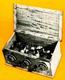
If you were under the impression that radio kits are a modern innovation, here's proof to the contrary. The 1924 Freshman Masterpiece kit above, a five-tube TRF model, was the pride and joy of the electronics hobbyist of that era. All three dials had to be adjusted to tune in a broadcast station.
