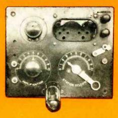
The first one-tube battery receivers used the WD11, a 1½-volt triode. This is RCA's Radiola which came shortly after Westinghouse's Aeriola receiver.
