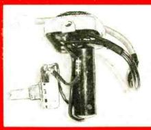
The adapter is shown removed from the can To install, first feed pot shaft through hole in can, then tighten nut
