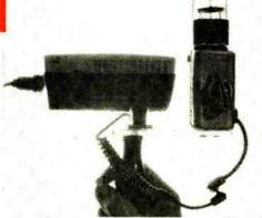
All it takes is a triggering flash to set the slave strobe off. Adjust potentiometer R2 for best sensitivity.
