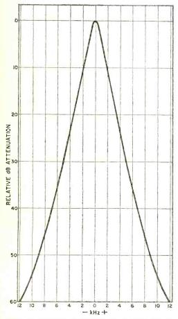
Clean symmetrical selectivity curve of the R-195 results from the use of ceramic filters in the i-f stages. Unfortunately, good selectivity cannot be used to maximum advantage due to poor bandspread.
