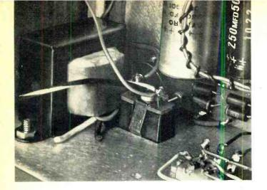
Input and output jacks J1-J4, ac receptacle SO1, and power transformer T1 are mounted on rear apron of chassis as in interior (above) and exterior (right) views. Strain relief protects line cord from sharp edges of entry hole in apron.
