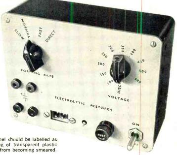
The finished front panel should be labelled as shown here. A coating of transparent plastic spray keeps lettering from becoming smeared.
