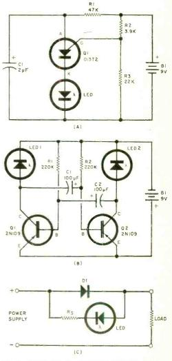
Fig. 1. Circuit (A) is relaxation oscillator blinker, (B) is dual blinker, and (C) is polarity reversal alarm, all using unusual light-emitting diodes.
