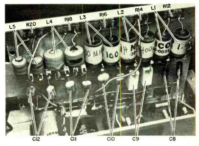
Capacitors, inductors, and resistors for filters mount on front panel of chassis. Terminal or tag strip is used to provide interconnection points for components.
