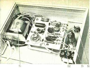
Interconnecting wires from chassismounted components can be soldered to appropriate points on the circuit board through use of "flea" clips.
