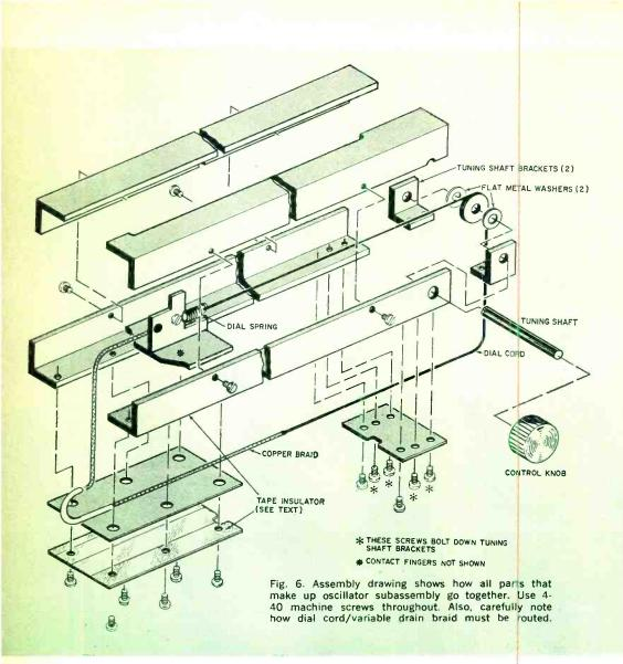
When properly put together, circuit board assembly should move freely in the chassis rails. Use just enough spring tension to prevent dial cord from slipping when you tune back and forth along the dial train.
