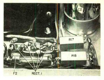
the power supply (see Fig. 4). Now, referring to Fig. 3, wire together the power supply circuit, using #18 or larger stranded hookup wire. (Note: Where #18 or larger wire is specified, do not substitute a smaller size wire. The circuits to which these wires connect carry as much as 10 amperes when the amplifier is driven to full power. If too small a wire size is used, power will be sacrificed and damping will suffer.)
