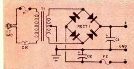
Fig. 3. Negative dc supply voltage is taken from right side of F2. Table lists ratings of F1 and T1 for desired amplifier output.
