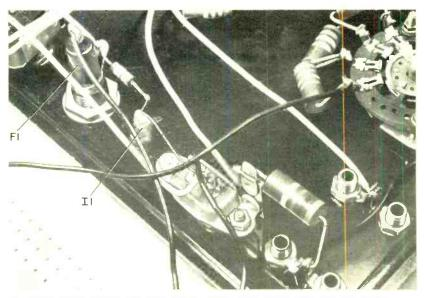
Be careful when drilling the holes in the plastic front panel as it will chip easily. The neon indicator lamp is cemented in the hole, other components use hardware.
