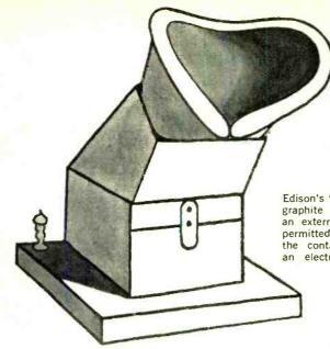
Edison's "black box" 1881 demonstration had graphite points which could be connected to an external circuit. The extension eye-shade permitted viewer to see, jumping between the contacts, sparks unlike any known to an electrical phenomenon at that period.
