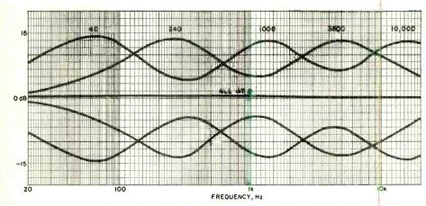
Response of equalizer at maximum and minimum settings; at zero position, response is flat.
