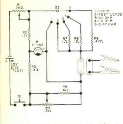
Fig. 1. Resistor R8 provides optional but very useful internal testing facility for checking calibration; S1 is momentary-action switch.
