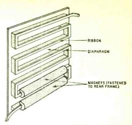
The Ge-Go "Orthophase" speaker had a long folded ribbon fastened to rear of flat diaphragm with a grooved magnet assembly interleaved with ribbon.
