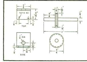
Fig. 5. Two short lengths of aluminum angle serve as supports for dial shaft. Faucet washer is cemented to shaft and grooved to make pulley.
