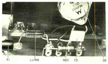
Fig. 5. Close-wind a single layer of #22 enameled wire along the entire length of R19 and solder the wire ends to the resistor leads to make the L1/R19 assembly.
