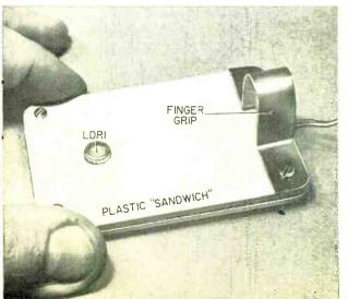
A simple plastic "sandwich" provides a convenient means of mounting light dependent resistor LDR1.
