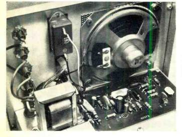
Behind the panel of the 150, wiring is very simple. Audio amplifier is assembled on a printed circuit board. Power transformer is at lower left.
