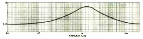
New curve was obtained with all controls set at zero, except 1000 Hz control set at +12 dB.
