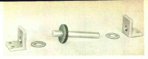
Shown is correct sequence of assembling parts that make up dial tuning assembly. Flat metal washers are used to reduce friction and wear between pulley and support brackets and to prevent play between them.
