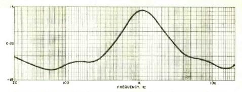
This curve was obtained with all controls set at -12 dB, except 1000 Hz control at +12 dB.
