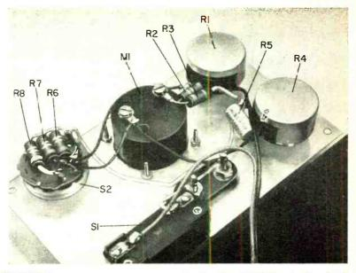
Fig. 2. The simplicity of the circuit allows all components to connect directly to the control and meter lugs.
