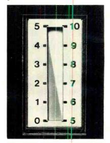
Two hundred microampere meter on new 150 is "different." Wired to collector of the audio output stage, the speaker had to be blasted to get reading half-way up scale. It looked like cat's eye.
