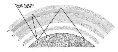
Signals may be reflected by a layer of the ionosphere or escape into space. Range is determined by layer height and wave angle.
