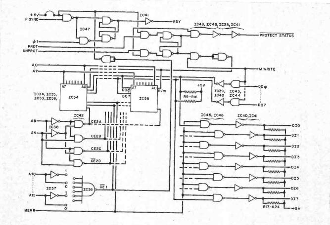
Fig. 5. The basic memory contains up to eight 256 x 4 RAM's.
