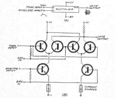
Fig. 4 (A) are typical connections for 4-quadrant multiplier. Key internal circuitry is shown at (B)
