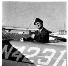
Antenna, on plane's fuselage, is cut for channel 13.
