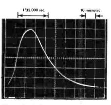
We used a high-speed oscilloscope to check flash duration of the Braun 2000, set to give briefest flash of 1/32,000 s. Measurement from pulse width at half height.
