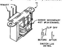
Fig. 3. Add a winding and terminals to the transformer and alter switch lugs as shown.
