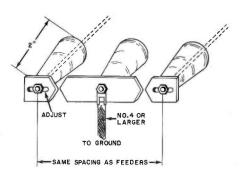
Fig. 1. A spark gap arrestor to protect ham antenna is easily made.
