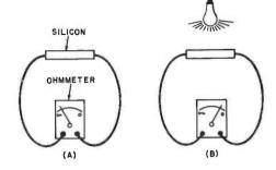
Fig. 6 With normal light on piece of silicon (A), resistance is high.
