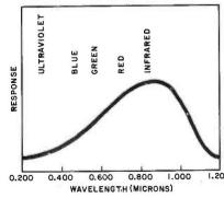
Fig. 7 Spectral response of silicon to various colors of light.
