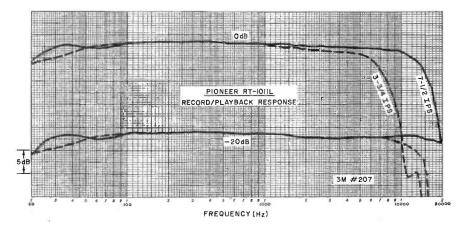
corder to be very accurate at both speeds. It was within ±0.5 dB from 50 Hz to 15,000 Hz at 7½ ips and within ±0.8 dB from 50 Hz to 7500 Hz at 3 3/4 ips. (These are the frequency limits of the test tapes.)
