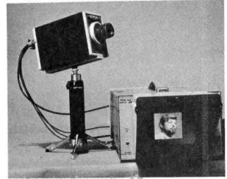
Fig. 3. Solid-state imaging system using a 50 by 50 sensor array. The image can be seen on CRT in front.
