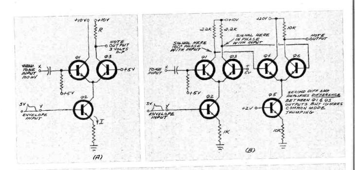
Fig. 3. In basic differential amplifier (A), envelope causes thump in the output. An additional amplifier can be added (B) to eliminate thump. Second stage can be an ordinary 741 operational amplifier.
