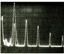
Fig. 5. Top (A) is output of one channel of FM tuner with 1-kHz signal. Spectrum analysis (below) shows 42-dB channel separation.
