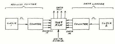
Fig. 2. Block diagram of pseudo-random data loader.
