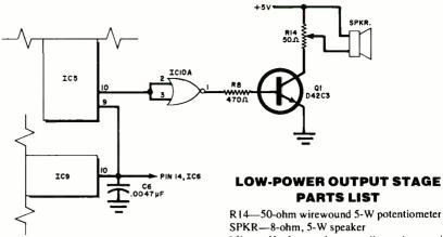
Fig. 2. Output stage for the low-power version.
