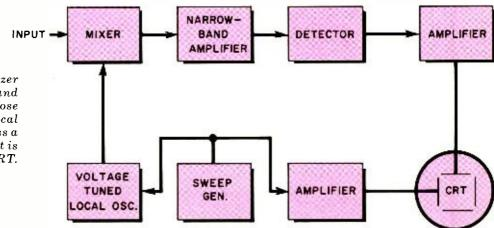
Fig. 2. A swept spectrum analyzer is basically a narrow-band superheterodyne whose voltage-controlled local oscillator is swept across a narrow frequency. Output is displayed on a CRT.
