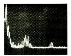
Fig. 8. Analysis of FM tuner has 1-kHz modulation signal followed by harmonics. Also shown are 19-kHz pilot carrier, its modulation products, and 38-kHz signal leakage.
