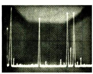
Fig. 2. Spectrum analyzer display of composite stereo modulation, with 100% modulation at 2000 hertz.
