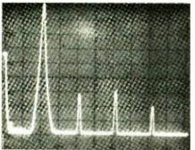
Fig. 3. Harmonics don't show in scope photo (A, top) of 1-kHz sine wave, but they do in photo of analyzer display (B, bottom).
