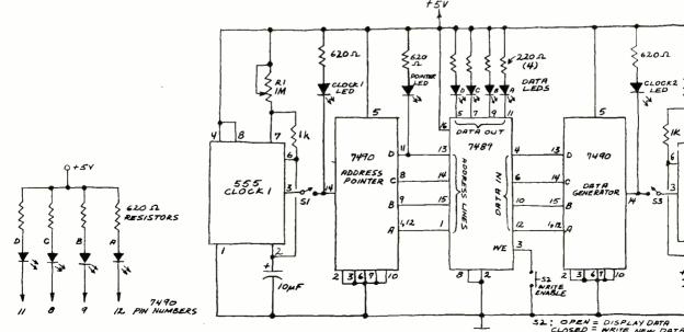
Fig. 1. Circuit indicates address pointer output.
