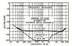
Frequency response and crosstalk with optimum tuning in and out.
