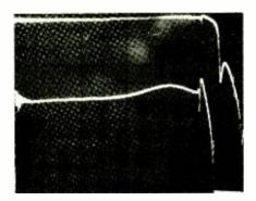
symmetry and rise-time characteristics. The same signal, viewed on the spectrum analyzer scanning from 0 to 10 kHz (Fig. 4B) shows higher than theoretical amplitudes for the 3rd, 5th, 7th, and 9th harmonics, and the presence of all even harmonics (which should be entirely absent in a true square wave) at a level of about -30 dB, or 3%, relative to the fundamental frequency. The even harmonic content shows a lack of symmetry in the square wave, which is not easily seen in the scope photo.
