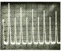
Fig. 4. Spectrum analyzer (B, bottom) shows undesirable even harmonics in square wave which appears clean on scope (A, top).
