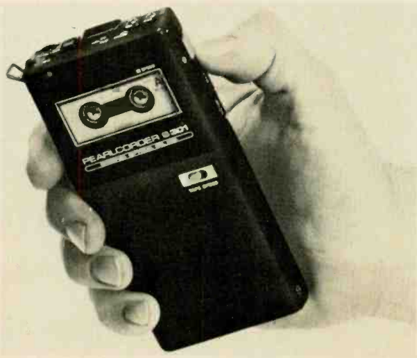
The most portable tape formats are the new "mini" and "micro" tapes, used in machines like this Olympus Pearlcarder.
