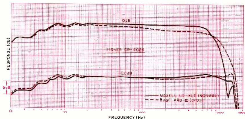
Frequency response for two types of tape at 0 and -20 dB.
