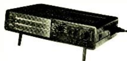
Fig. 2. Nakamichi T-100 Audio Analyzer has plasma readout.
