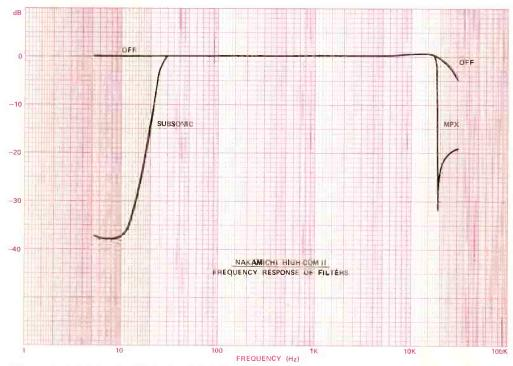
Frequency response curves with the filters off is flat within  $\pm$  0.6 dB from 5 to 20,000 Hz. The subsonic filter cuts off below 30 Hz, and the MPX filter notches at 19 kHz.
