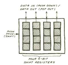
Fig. 8. Four 4-bit words can be stored in this memory stack.
