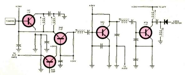
Fig. 2. Partial schematic of the automatic gain control circuit and four-stage video i-f strip.
