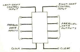
Fig. 4. Inputs and outputs for a hypothtical universal four-bit shift register.
