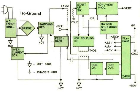
Fig. 3. Block diagram of the power supply system showing how two ground points (hot and chassis) are used.
