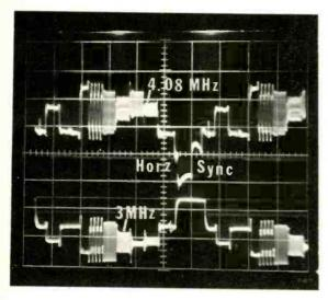
Fig. 6A. At top is multiburst at the video detector's output. Bottom trace shows that luminance bandpass allows only 3 MHz to reach the CRT.
