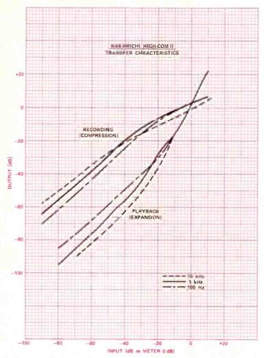
Static input-to-output transfer characteristics of High-Com II showing compression and expansion at frequencies of 100 Hz, 1 kHz, and 10 kHz.
