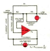
Fig. 5. Another inverting op-amp circuit where unknown resistance forms amplifier's input resistor.
