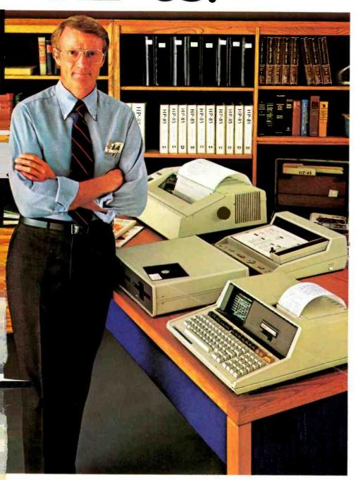
The Personal Computer For Professionals: HP-85 specifications: Memory—16K RAM expands to 32K, 32K ROM expands to 80K; CRT—32 chars./line, 16 lines; graphics—256 X 192 dots; thermal printer—2 lines/sec.; magnetic cartridge capacity—200K; I/O—HP-IB (IEEE 488), RS-232, 16-bit GP-IO, BCD; Application Pacs include Statistics & Regression Analysis, Finance, Math, Linear Programming, Text Editing, Waveform Analysis, Circuit Analysis, BASIC Training, & Games.
