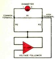
Fig. 3. Here, the voltage follower prevents shunting components from influencing theohameter reading.
