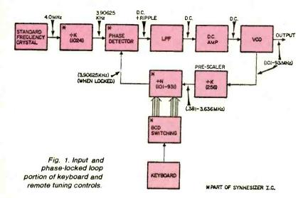
tems without channel scan have 10 keyboard command buttons for selecting any vhf or uhf channel. (Single-digit channel numbers must be keyed in preceded by zero, such as 02,03,04, etc.) Receivers with up/down channel scan have 12 buttons. Neither type of channel-selection system has receiver or remote programming for channel scan; stations must be sequenced in strict up or down numerical order.
