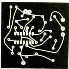
Fig. 5. Actual-size etching and drilling guide for a printed circuit board for the Infrared Road Icing Alert is shown above right. Component layout above left.
