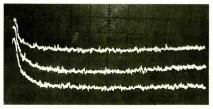
Composite spectrum-analyzer photograph of response from 0 to 20,000 Hz with no noise reduction (top), with Dolby B (center) and with High-Com II (bottom). Dolby B reduces noise by 9 to 10 dB, High-Com by about 12 dB more.
