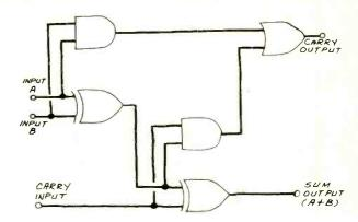
Fig. 5. Logic diagram of a binary full adder.
