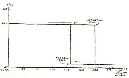
Fig. 2. Switching action, showing hysteresis, of a UGN-3020T.
