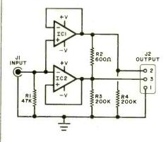
A. The circuit shown in the figure should work well for you. Two op amps functioning as voltage followers are employed. One follower (IC1) delivers a noninverted version of the input signal, but the other (IC2) inverts it. The outputs of the op amps appear across R2 180° out of phase with respect to each other and are applied to the signal-carrying terminals of balanced connector J2 (Cannon XLR-3-13 or equivalent). Resistors R3 and R4 reference the "hot" output terminals to system ground.
