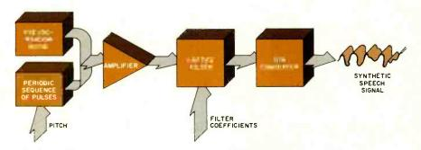
Fig. 1. The excitation signal for Texas Instruments' speech synthesizer system can be periodic impulses for voiced sounds or pseudorandom white noise for unvoiced sounds. Data needed to select type of excitation, determine degree of amplification, and specify filter coefficients is stored in ROM.
