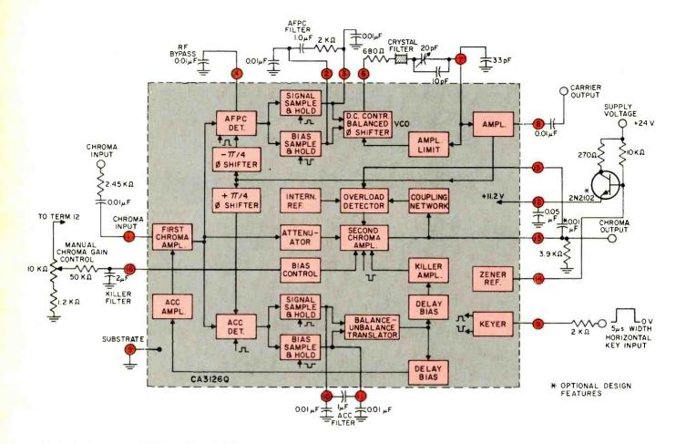
Fig. 5. Block diagram of IC600, an RCA CA3126Q chip which makes up the complex chroma processor circuit.
