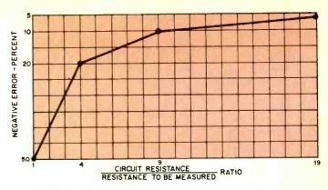
Fig. 1 Graphical analysis of the error in a resistance measurement caused by uncompensated shunting circuit resistances.
