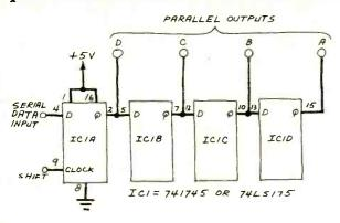
Fig. 3. A four-bit shift register made from a single quad D flip-flop.
