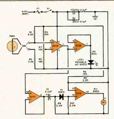
Fig. 4. The thermistor is part of a bridge that drives comparator IC1A. When this comparator tums on (detected temperature below preset), it activates a LED and an audible alarm.
