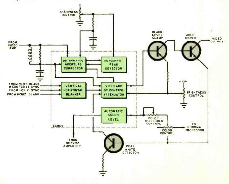
Fig. 4. Diagram showing operation of the IC900, the video clamp/processor and color amplitude noise limiter.
