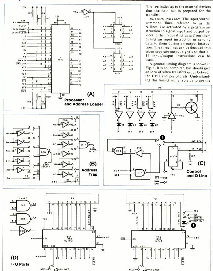
Fig. 5. The various parts of the circuit on the Product Board are shown schematically above and on the opposite page. Numbers in circles indicate jumper pads.
