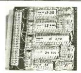
OK Machine and Tool Corp. is now offering the "Socket-Wrap I.D.," an identification system designed for use with wrapped-wire IC sockets. This system comprises a number of socket-
