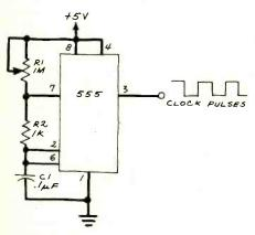
Fig. 3. A 555 clock pulse generator.
