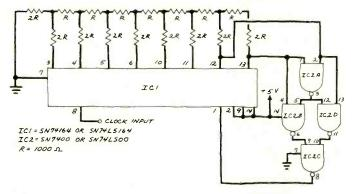
Fig. 2. Schematic of a pseudo-random voltage generator.
