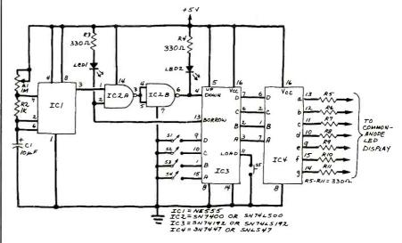
Fig. 1. Schematic diagram for a programmable countdown timer.
