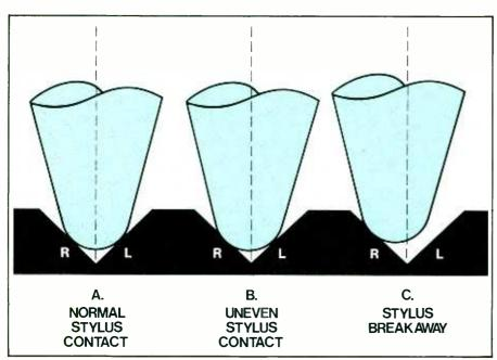
Fig. 3. Varying conditions of contact between stylus and record groove. In soft mistrack (B), stylus force is unevenly distributed between groove walls.
