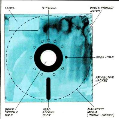
Fig. 1. Configurations of a 51/4" (above) and 8" (opposite) diskettes as used in small computers, with makeup of a diskette at far right.
