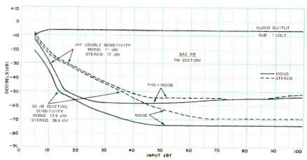
Noise and sensitivity curves for FM section of the SAE H9 receiver.
