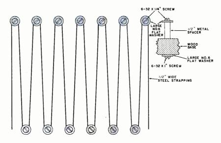
Fig. 2. Using this diagram as a guide and following instructions in the text, you can make up your own load resistor from ½-inch steel banding strap.
