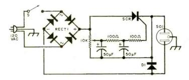
would be disasterous, such as drilling holes in a finished front panel or project enclosure. Medium-speed drilling is often employed when working on nonferrous metals such as aluminum and brass. The circuit presented in the figure will allow you to vary the speed of a standard fixed-speed drill without performing any modifications to the tool.
