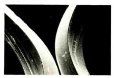
Fig. 6. Electron micrograph of a mistracked groove shows ruts caused by errant stylus.
