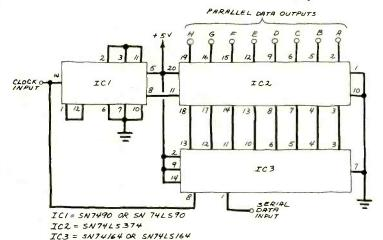
Fig. 4. Schematic of an 8-bit serial-to-parallel data converter.
