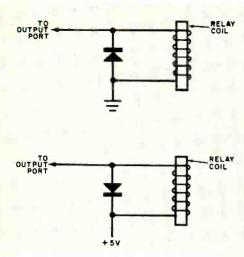
Fig. 6. How to determine load resistances on output ports. In circuit above, minimum relay coil resistance is 2.1 k $\Omega$ . The relay is active when the output is high. In the lower circuit, minimum relay resistance is 820 $\Omega$ . The relay is active when the output is low.
