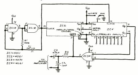
Fig. 1. Schematic diagram of a pseudo-random sequencer made from CMOS shift registers.
