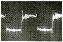
Fig. 1. Oscilloscope trace (above) of cartridge output from a 1-kHz square-wave band of a CBS STR-112 test record. "Ringing" at 41 kHz is evident. Fig. 2. (right) shows an electron micrograph of the test record groove. Note how the ripples in the groove correspond to the "ringing" signal observed in Fig. 1.
