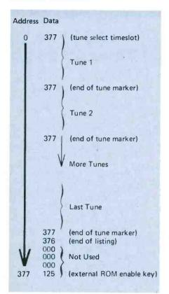
Fig. 4. PROM memory allocations for a simple programming example.
