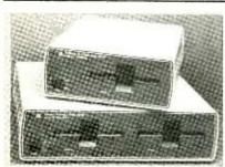
The HP 82900 Series disk drive from Hewlett-Packard reads double-sided, double-density 51/4" diskettes and can be configured to provide from 270K bytes to 1.08M bytes of storage for the HP-85 Personal Computer. With its interface, the HP-85 Mass Storage ROM (\$145), plugged into the HP-
