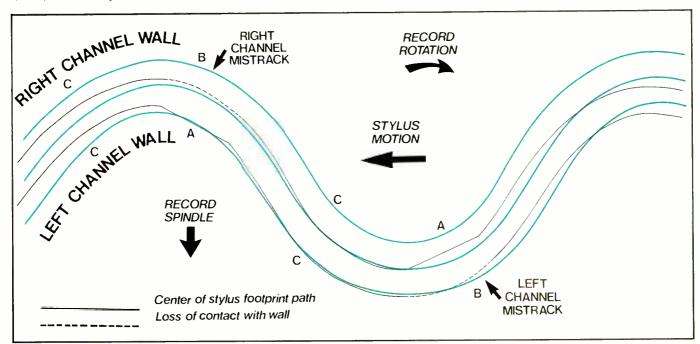
Fig. 5. Mistracking of a monophonic sine-wave groove.
