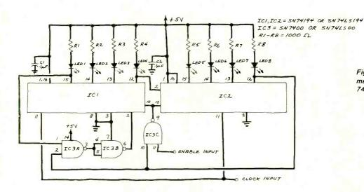
Fig. 6. A bargraph generator made from a pair of 74194 shift registers
