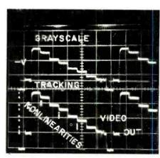
Fig. 5. Grayscale tracking reveals that eight steps are somewhat erratic though horizontal portions are fairly even.
