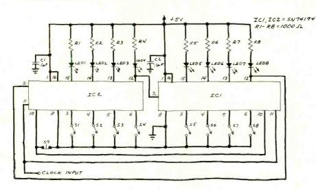
Fig. 5. A shift-register 8-bit programmable sequence generator.
