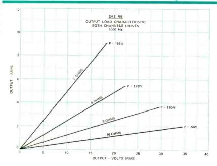
A voltage-current plot of the output characteristics at clipping of the SAE R9 for various load impedances. Maximum open-circuit voltage is about 34.4 V; current in excess of 9 amperes to a low-impedance load trips protective system. Both channels driven by a 1-kHz signal.
