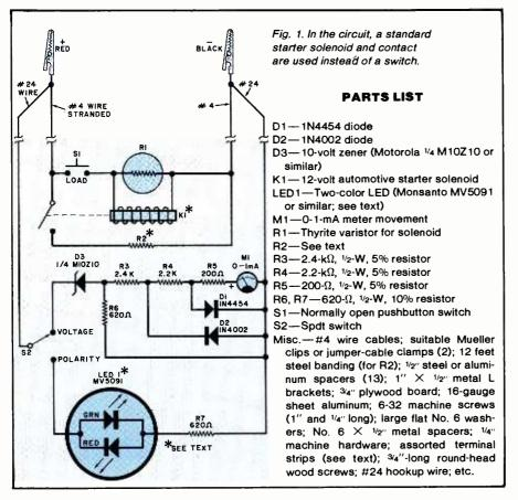
and diodes D1 and D2 make up a 0-to-6-volt de voltmeter. When connected in series with 10-volt zener diode D3, this meter circuit becomes an expanded-scale 10-to-16-volt de voltmeter. Diode D2 protects the meter against reverse polarity, while diode D1 protects against overvoltage when the meter is connected in proper polarity.
