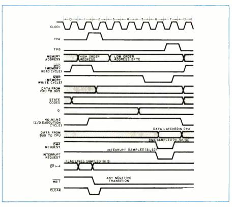
Fig 4. The timing diagram is used to show signal relationships. Shaded areas indicate undefined state when multiple transition may occur.
