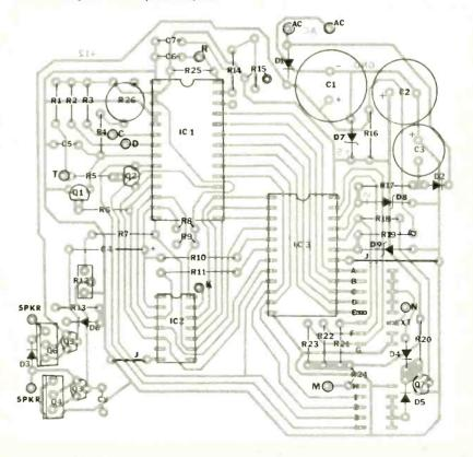
careful to observe the polarities of diodes and electrolytic capacitors and lead locations on the transistors. Do not install the ICs in their sockets until told to do so in the following procedure.
