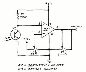
Fig. 3. An expansion of the circuit in Fig. 2. using an operational amplifier for higher gain.
