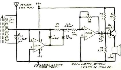
Fig. 2. An AM radio using an operational amplifier.
