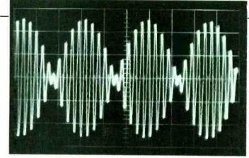
Fig. 1. Oscilloscope photo of the alert signal of the Emergency Broadcast System. It consists of two tones at 853 Hz and 960 Hz broadcast for 22.5 seconds.
