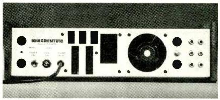
Rear panel of C4P with I/O ports.
