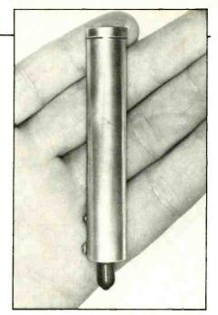
Fig. 6. A battery-driven miniaturized single-heterojunction laser transmitter.
