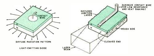
Fig. 1. Comparison of the physical structures of a light-emitting diode (left) and a simple diffused-junction laser.
