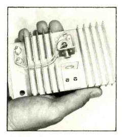
Fig. 7. A DH laser with collimating lens installed on an oversize heat sink.
