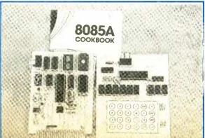
The 8085AT single-board computer from Paccom can be used as a controller or trainer. gent modems designed to fit any computer with a serial interface. Prices for the Bizcomp units range from \$395 for the model 1030 to \$495 for the 1031.
