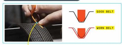
Poly-V belts seem to last a lot longer than the old-fashioned V-belt ever did. It's not unusual for a belt that uses a springloaded automatic tensioner to last 100,000 miles or longer. But like any moving part, these belts eventually wear out too. It's easy to see some of the signs of imminent failure, like weatherchecked rubber or the dangling strings of the reinforcing fabric whipping around. These both mean it's time to
