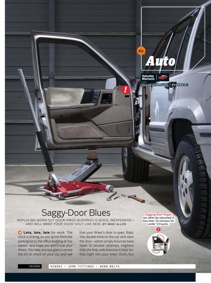
try a kinder, gentler slam, and realize the end of the door has sagged a good inch from its original position. The only way to close the door is to use both hands on the handle (chipping a fingernail) and lift the 75-pound door up until the latch matches the height of the door striker, and then bump it with your
