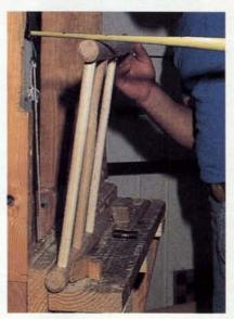
6 MORE EYE-BALLING • Loosely clamp the front legs to the bench with the spokes pointing up from the shelf at a 90 degree angle. Now rotate the upper front leg toward you 2" (which is half of the difference between the length of the front spokes and the length of the side spokes). This creates the necessary angle for drilling the front
