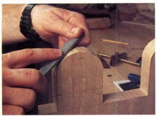
CRITICAL TENONS • Here I'm shaping the tenons with a rasp after I roughed them out on a band saw. Notice the pencil marks on the tenon. The two dark lines show where the side will go on the tenon. Note that the location of the mortise is a little inside that line. This pulls the whole table tight when the wedges are inserted.
