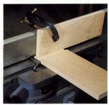
Tenons are back-to-back rabbet cuts. Because they're run against the grain, some tear-out can occur at the ends of the cut.
