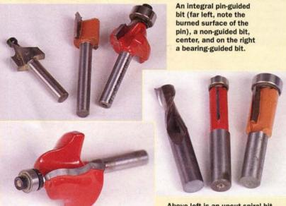
The anti-kickback design offers a much smaller gullet space to avoid anything being trapped between the wings. The extra material also improves the stability of the cut. Above left is an upcut spiral bit, which is excellent for removing waste in moritse operations; center is a straight flush cutting bit; and on the right is a shearing flush cut bit for cleaner, easier operations with dense or highly figured woods.
