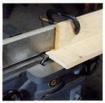
2A tongue is formed by inverting the stock and making a second pass. Adjust the clamped hold-down block to suit.
