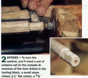
spindle gouge and an awl. In this photo, the 1" flat chisel is shaping the tenon to the final dimension (top). After the tenon is cut, flatten the sides of the tenon with a whittling knife to keep the mortises from splitting.
