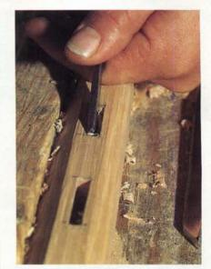
HAND-CUT MORTISES • With the mortise locations marked, put the front legs aside and start cutting the mortises in the back legs first. The rectangular mortises for the slats are 1/4" wide x 1" deep and should have a flat bottom. These mortises are marked out on the quarter grain, so they will run parallel to the growth ring, and then chopped out with a 1/4" mortising chisel in line with the growth rings. After chopping out the general shape. clean up the sides with a 1" flat chisel.
