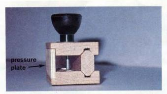
3 ADD PRESSURE PLATE • Cut the pressure plate and glue it into the rabbet in the top plate. The fence will still work if the pressure plate is glued into both rabbets, but you'll have to remove the guide rail to clear the table for freehand work.
