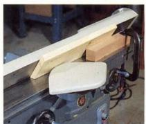
The jointer makes perfectly smooth bevels and chamfers. I prefer to work with the fence at an acute angle (less than 90 degrees).
