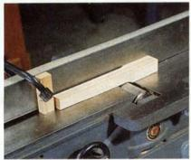
A leg shape that needs to be reduced in size for a limited length is a straightforward chore for the jointer. The work is placed on the infeed table and moved forward until it contacts the stop block. Then the cut is repeated on the remaining three sides.
