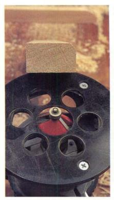
CHAMFERS ALL OVER . Chuck a chamfer bit into your router and cut a 1/4" x 1/4" chamfer on the outside edges of the piece that aren't part of the joinery. Shown here is the chamfer cut on one edge of the end cleat.
