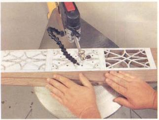
SCROLL SAW TIME . Cutting through 1" walnut on a scroll saw can be a little taxing. Choosing the proper blade for this task can make things a lot smoother (I recommend a 5R or reverse-tooth blade with 12 teeth per inch). The length of the sides can be problematic for maneuvering on the scroll saw, but the end effect of a single pierced piece is worth the effort.
