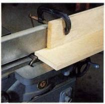
I use the jointer for rabbeting more than any other machine. Cuts are smooth and precise and the machine is easy to set up for the chore. A clamped block helps keep the work flat on the table. Because you have to remove the guard, be especially careful with where you put your hands.
