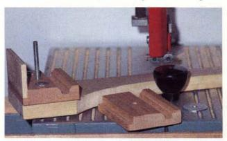
2 BUILD THE CLAMP • Cut the <sup>3</sup>/<sub>8</sub>" x <sup>3</sup>/<sub>8</sub>" groove first, then mount a 1"-diameter 45-degree chamfer bit and cut the chamfers without moving the fence, so the alignment will be perfect. Again, use multiple passes to form the chamfers. Test fit the rail in the groove while the guide rail is bolted to the band saw table. The board's top surface should be about <sup>1</sup>/<sub>8</sub>" above the table.
