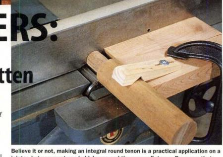
Believe it or not, making an integral round tenon is a practical application on a jointer, but you must use hold-downs and the proper fixtures. Be aware that the guard isn't used for this technique so be careful.
