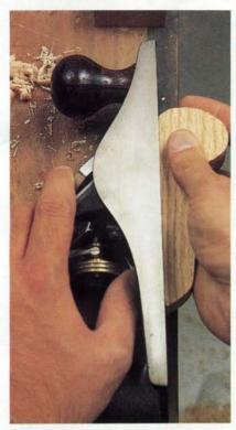
SIZING WEDGES · The wedges in the PullOut Plans are a little oversized, so you'll have to cut them down a bit to get a snug fit. The best way to do this is to run them flat against a bench plane that you're holding down against your work bench. Take light passes on the back and sides. then try to fit the wedge into the mortise. Continue shaping until the wedge pulls the joint snug. If the round head of the wedge is touching the tenon, then you've cut your wedges too small. Start again.
