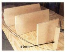
SHELVES IN PLACE . Here you acan see that the shelves I cut fit inside the layout of the "hull" on the plywood. Note that I was still planning to use a curved bow at this stage. I soon gave this up and opted for straight-sided shelves.
