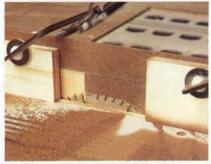
MAKE YOUR OWN SIDING • I made this simple jig to safely and accurately cut the bevel on the hardboard siding. Sandwich a scrap piece of hardboard between the two plywood pieces to create the opening through which you push the long strips of siding. Set your table saw to cut a 7-degree angle and run the hardboard through the slot.
