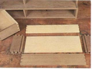
DRAWERS • The drawers for this shelf were assembled using half-blind dovetails cut with a dovetail jig. If you have the time on your hands, you also can cut these by hand. And if you're not entirely comfortable with dovetails, you can always use tongue-and-groove joints to assemble your drawers.
