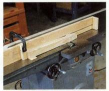
A companion taper to complete Othe leg shape is formed the same way. In this case use two stop blocks. Brace the work firmly against the front stop block before you lower it for the cut. A small nail, tapped in the aft end of the stock will make the leg easier to pull across the knives.
