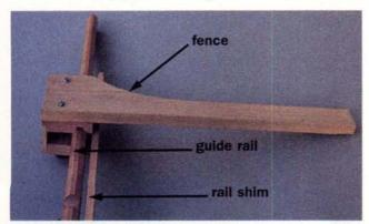
1 PREPARE THE GUIDE RAIL • Here's a top view of the fence. The guide rail and rail shim run through the clamp in the middle of the photo. Lay out the bolt hole locations on the rail, then clamp the guide rail and shim together and drill the appropriate clearance holes through both. Mark the location of the miter gauge slot and cut an oversize notch that clears the miter gauge's guide bar, then bolt the rail and shim to the table.
