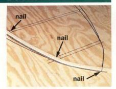
MAP THE BOTTOM . Start at the stern. Place the stick to the inside of the nail, then bend it around the outside of the nails at the other shelf locations, then inside the nail at the bow. Draw a pencil line following the stick. Repeat the process for the other side.
