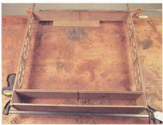
A DRY FIT • With the dadoes made on the sides, cen-2 ter partition, top shelf and drawer section top and bottom, dry-fit the shelf unit and use a 1/4" rabbeting bit in a router to form the rabbet for the 1/4" back in the drawer section. Chisel out the corners to complete the rabbet.
