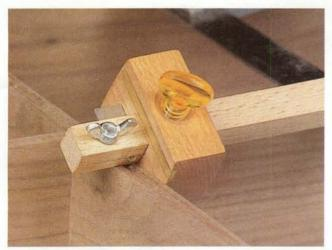
3 HANDMADE DETAIL • I used a beading tool to add the flute detail to three front edges. Any number of details can be used, or none at all if that's your preference. If you've never used a beading tool before, it may take a couple of minutes to get the feel of the cutting action. Take it easy and let the tool cut a little at a time.
