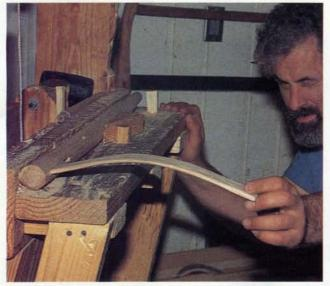
4 FINDING THE RIGHT ANGLE • Loosely secure the back leg in the vise with the opening of the slat mortises facing toward you. The front of the leg is down. To get the correct angle for drilling the mortises, place one of the slats in its mortise and slightly rotate the leg up until the slat is in the proper position with the line of the back of the chair parallel to the bench. This takes practice and careful eye-balling.
