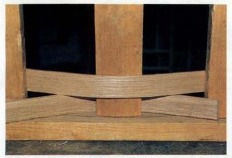
BENDING JIG . If you're working with dried wood, the pieces will need to be soaked for a few days, or put in a steamer prior to bending.
