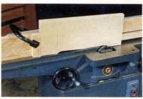
8 This photo shows a recessing cut with only the infeed table lowered. The second cut is made after reversing the stock's position.
