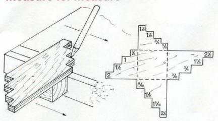
I've been using notched pieces of wood as pencil gauges for years. I found there were some measurements I needed frequently, so I made a block with several sizes, and eventually made a single gauge to incorporate all the sizes I commonly use.
