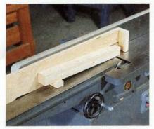
Form short tapers by bracing your leg against a stop block and pulling it across the knives. Use a hold-down to keep the work in place as you pull it for the cut. Always keep the guard in place, even though it isn't shown in these photos.
