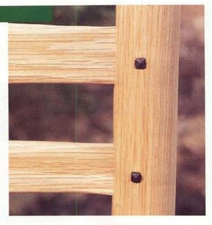
Chair Assembly • To assemble the chair, first glue one set of spindles in one of the front legs. Place the spokes in the mortises with the flattened sides of the tenons running parallel to the leg length.
