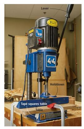
Hollow-chisel mortisers excel at boring square holes. Here you can see the holddown (which is usually inadeguate with other machines), the table (which must be squared to the chisel before use) and the lever (which makes the machine plow through almost any job).
