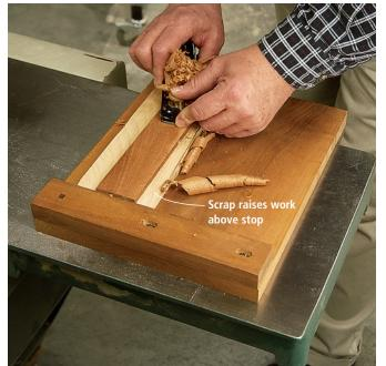
Bench hooks can be used almost anywhere (such as on the bed of this jointer) and can do some surprising tasks. Here it is being used as a small planing board. The light-colored scrap below the work raises the work above the bench hook's stop.
