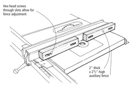
To attach the fences, I used  $\frac{1}{4}$ " x  $2\frac{1}{2}$ " self-tapping hex-head screws that I can easily loosen and tighten with a nut driver.
