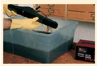
After attaching the negative lead to the piece of rusted metal, attach the positive lead to a sacrificial piece of metal. Then place this object in the bucket a few inches away from the rusted piece. After a while, remove the objects and see how much rust is gone. We think you'll be pleasantly surprised.
