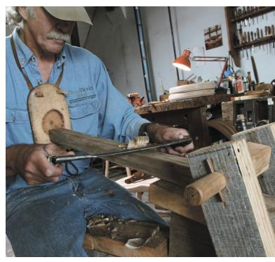
The drawknife can be used with the cutting bevel up or down. When making a planing cut like this one, I skew the drawknife and use the tool bevel-up. I'll use it bevel-down for tight work, such as for shoulders on rounded tenons.
