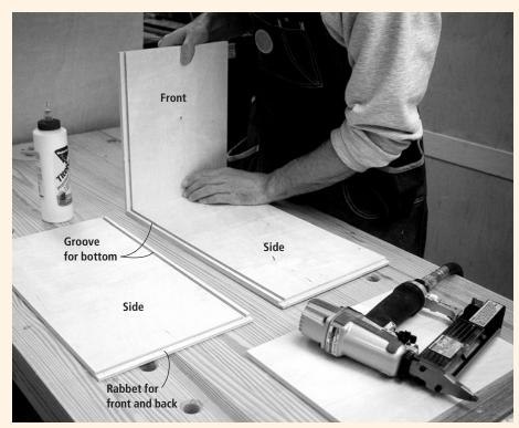
This drawer box is made pretty easily with rabbets. The front and back rest in  $\frac{1}{2}$ "-wide x  $\frac{1}{4}$ "-deep rabbets in the side pieces. The bottom slides into a  $\frac{1}{4}$ "-wide x  $\frac{1}{4}$ "-deep groove in the sides and front. The back is  $\frac{1}{2}$ " shorter than the front to allow the bottom to slide in.
