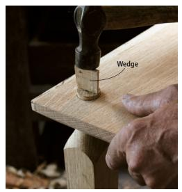
The wedges lock the legs in place and tighten up the fit between the tenon and its mortise.
