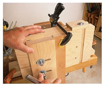
Switching the jig for end mortises is a matter of removing the horizontal workrest and replacing it with the vertical one. Clamp a rail to the jig with its centerline aligned with the jig's setup line to locate the workrest while you secure it. Nothing else changes in the setup.
