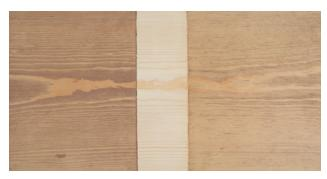
On this board, I applied a gel stain (left) and a liquid stain over a wood conditioner that had dried overnight (right). You can see that neither procedure adds much color to the wood, but both eliminate the blotching. Gel stain requires only one step, however, and wood conditioner followed by the stain requires two — and overnight drying in between.
