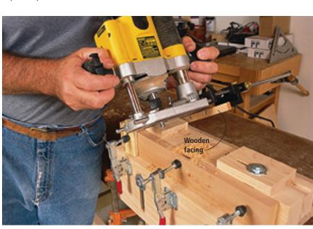
The wooden facing on the edge guide drops into the channel at the back of the jig, allowing you to move the router back and forth without worrying if it will wander off course. The stops control the router's travel, ensuring the mortise will be the correct length.
