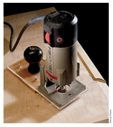
Making a Router Cut Like a Hand Plane
