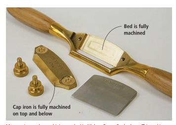
More praiseworthy machining on the Lie-Nielsen Boggs Spokeshave. This tool is a bit different in that the cap iron contacts the iron at more points than other tools. This adds stability to the iron, which allows for fine and coarse cuts.
