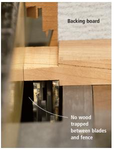
The second pass has the work against the fence and defines the face shoulder. Note there isn't any wood between the fence and blades, so the chance of kickback is minimal. The backing board reduces the chance of tear-out at the shoulders.
