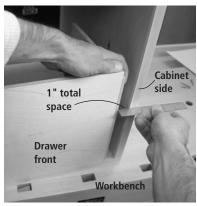
When building drawers with slides, the most critical dimension is the width of the assembled box. If you're off by more than  $\frac{1}{32}$ ", the slides won't work. It pays to mock up an assembled drawer to get the fit just right. Standard drawer slides usually need  $\frac{1}{2}$ " of space between the drawer and case, so shoot for a drawer that's 1" less than the total case opening.
