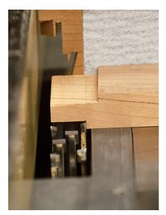
When making tenons with a dado stack in your table saw, the first pass should remove the bulk of the material. Keep firm downward pressure on your work, which will give you more accurate cuts.
