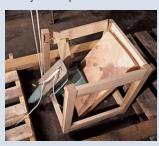
4) The mortise-and-tenon cube collapsed after the second hit.
