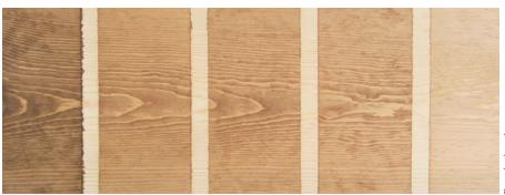
In the far left panel, I applied a liquid stain directly to the wood. I then applied a varnish-based wood conditioner to the rest of the board. I applied the same stain to the second panel immediately, the third panel after ten minutes, the fourth panel after two hours and the rightmost panel the next day. You can see that the blotching problem isn't solved unless the wood conditioner is allowed to completely cure.
