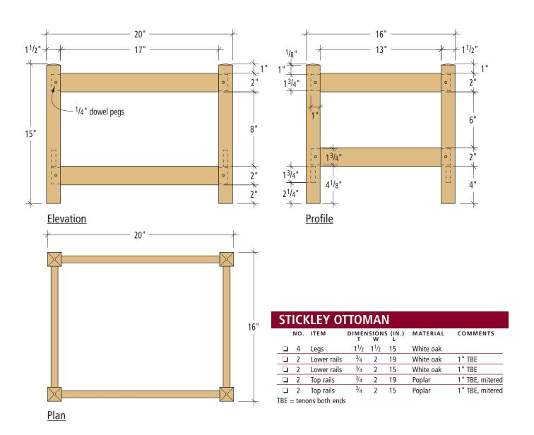
Just as with the test run, assemble the ends first, applying glue to the inside of the mortises, lightly covering all four walls. Applying the glue to the mortise rather than the tenon will keep glue squeeze-out (and clean up) to a minimum.
