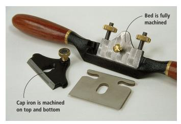
Now this is more like it. Note that the bed of the tool is fully machined. This is what you pay for with a premium tool such as the Veritas. The excellent fit between the body and iron translate into excellent cutting action. Also note the machining on the front edge of the cap iron. This helps the shavings escape.
