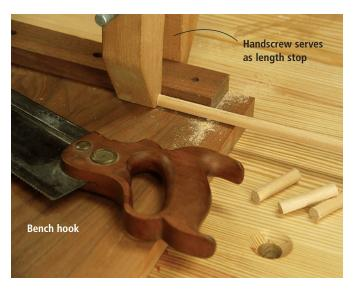
Cutting short pieces to accurate length is a tricky operation with a miter saw. The bench hook, backsaw and a handscrew clamp make the job safe and efficient.
