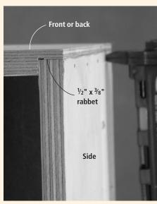
Joining drawer sides to the front and back can be as simple as cutting a rabbet. Then you can use glue and nails to complete the joint.
