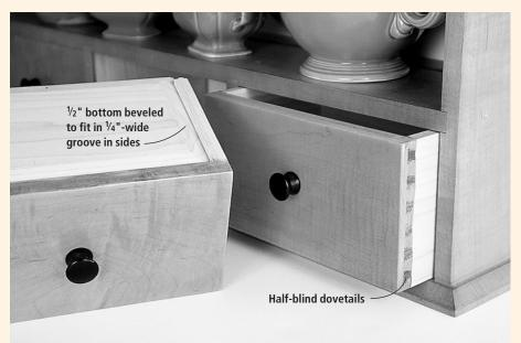
The drawer bottoms in the drawers shown at left are ½" thick but are beveled to slip into a 1/4" groove, a traditional drawer construction method. Also, you can see the half-blind dovetails connecting the side with the front.
