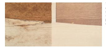
The liquid stain I applied (left) caused blotching, but the gel stain (right) didn't. You can see the deeper penetration in the blotched areas after a pass with a hand plane.
