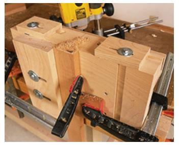
The rubber tips of toggle clamps have too much give, so I use deep-throat clamps to secure the work for end-mortising.
