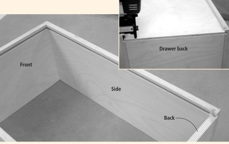
A simple drawer bottom is easily made from  $\frac{1}{4}$ " plywood. The sides and front of the drawer are grooved with a straight router bit,  $\frac{1}{4}$ " up from the bottom edge. The back is held short at the top of the groove. With the bottom slipped into the groove (shown in the inset photo), you can square up the drawer, then nail the bottom in place into the drawer back.
