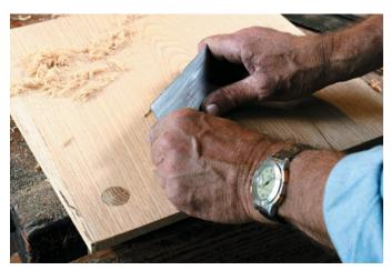
The simplest and most useful of tools, a properly tuned card scraper is the tool to use to prepare a surface for finishing at all stages of the project.
