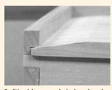
Traditional drawers used raised panels made of solid wood for the bottoms. These are easily made on a router table with a raised-panel bit, then fit into a standard groove in the drawer sides.
