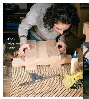
Use scraps as spacers to ensure that your leg assemblies go together just right. This is a lot easier than measuring everything. Then screw it together using stainless steel screws.
