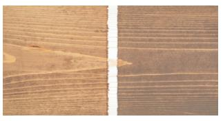
Liquid oil-based stain (left) causes considerably worse blotching than liquid water-based stain (right) because water-based stain is naturally thicker. As a result, depending on the wood you're using, you may be able to apply water-based stain without any blotching. But to be safe, do a test on scrap from your project.
