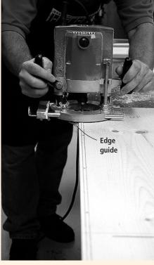
Rabbets and grooves are pretty easy to make with a hand-held router. Here you see a router cutting a  $\frac{1}{4}$ "-deep groove with a  $\frac{1}{4}$ " straight bit and an edge quide.
