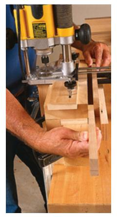
Here I'm cutting twin mortises. A spacer shares the channel with the edge-guide facing. With the spacer between the jig and the facing, the router can cut the first mortise. Moving the spacer behind the facing bumps the router out, so it can cut the next mortise.
