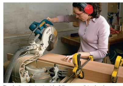
We used a miter saw to cut our pieces to length. Here you can see that we clamped all the top boards together and "gang cut" them to length simultaneously.
