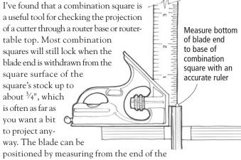
stock with an accurate ruler. The broad surface of the stock will stand steadily on an inverted router while extending over the bit opening. Percy Blandford
