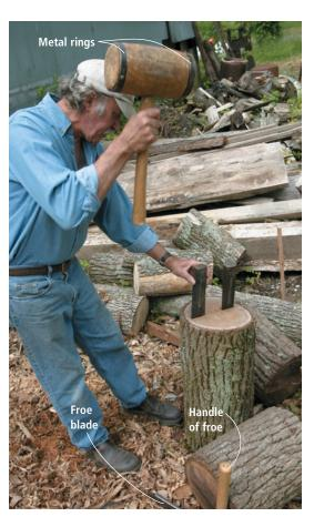
is a traditional "L"-shaped tool for splitting – or riving – green wood. Just drive the tool's wedge-shaped blade into the end grain and then work the wooden handle, pushing and pulling it to open the split. One of its charms is that it will follow the grain of your timber instead of cutting across it like a sawmill will. The result is a billet (a halved or quartered log, or roughly dressed lumber) with straight grain.
