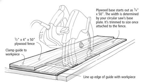
the panel, aligning the edges, then cut the panel to its final width by running your circular saw along the fence.
