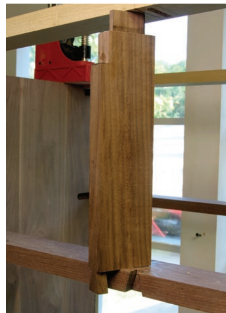
Want to make it easy? All the joinery work on the center divider is hidden—covered by the mouldings or the top. To make quick work of the divider, attach the piece to the blade and support rail with screws.
