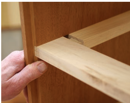
View from the back. Here is a the rear of a drawer web frame with the rear tenon's shoulder cut short and left unglued to accommodate movement of the solid wood case side.
