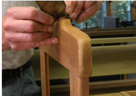
Final slices. A curved-edge card scraper efficiently removes the marks left by the rasp and removes any high spots along the edges.
