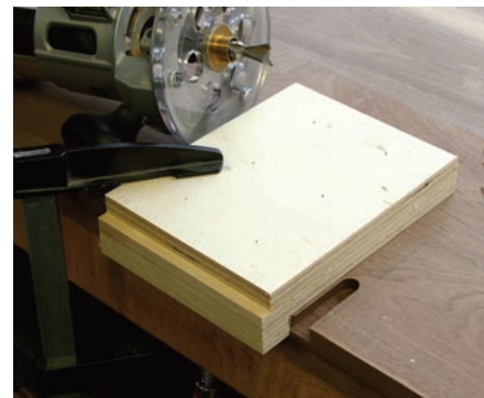
Best router setup. A platform jig, \frac{3}{4} "-dovetail router bit and a \frac{3}{4} "-outside-diameter guide bushing are used to create the sliding dovetails that attach the drawer blades to the case. It's simple.
