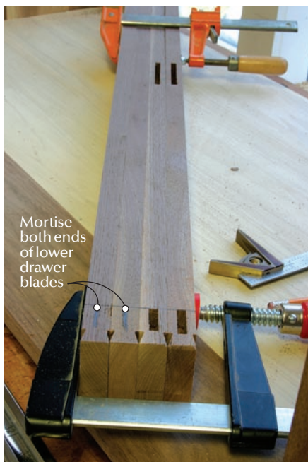
Strong connections. The top and rear blades are mortised for the housed and center runners. The lower drawer blades have a single mortise cut at each end to hold the runners in position.
