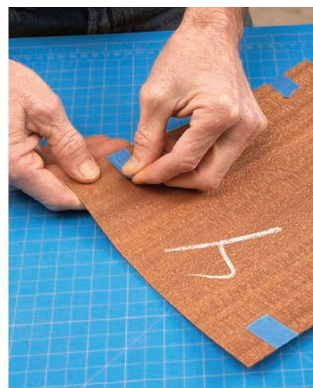
2 Stack it to be accurate. With masking tape, tape the entire bundle together to create a packet of veneer; this will keep each piece from shifting when cutting. I recommend that you stack cut all four pieces.
