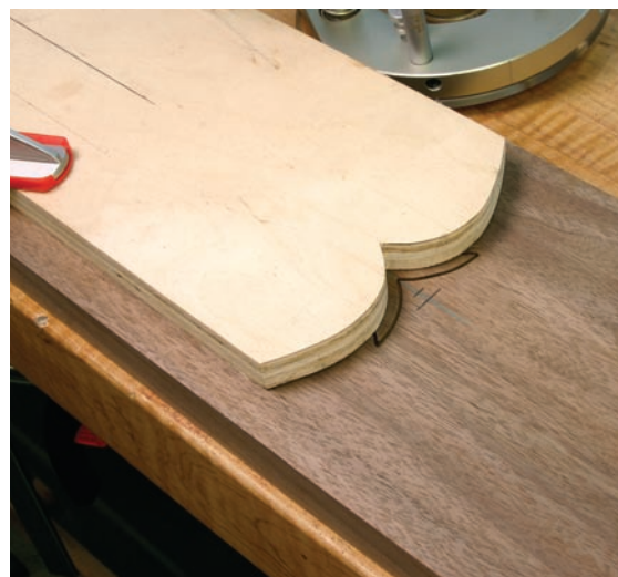
Plunge to begin. The tulip top string groove is the first of two grooves that require that you see the bit as you work – or develop a feel for when to stop at the line.
