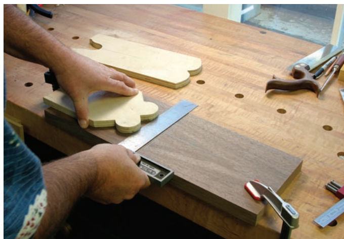
Keep it straight. The jigs used in this project are all held square to the drawer front. Proper placement is essential to the task.
