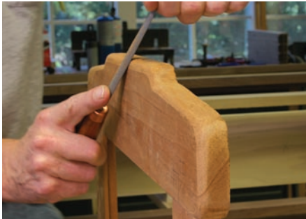
Variable curves. The radius of the rounded edges varies along the length of the edges. A series of rasps will allow you to go from rough to nearly ready in a short period of time.
