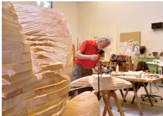
Steady work. Stacked laminations are cut to size from computer-generated patterns and clamped up rough before being carved to finished shape.
