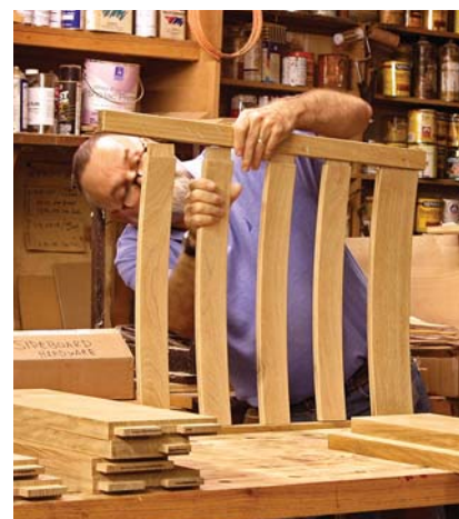
Just a minute. With experience, precision joinery is efficient. Final fitting of the joints in this chair back takes less than 10 minutes.
