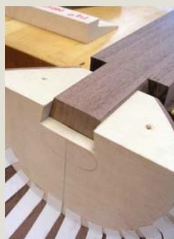
Joint under pressure. The oud’s bowl and neck are joined using a stout, perfectly fit dovetail. The joint must withstand hundreds of pounds of pressure from the instrument’s 11 strings.
