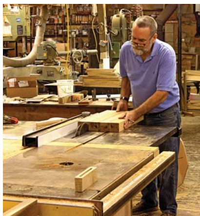
Four good sides. Dale has a unique method of making legs with quartersawn figure on all four sides, gluing four legs' worth of material at a time into a single block.
