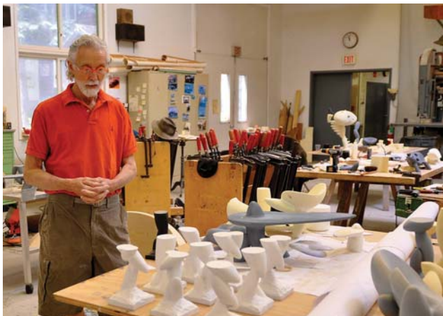
Technology at work. These days, models are carved from urethane foam and scanned into the computer, which then creates patterns for each layer of wood.
