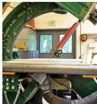
Giant saw. This boat builder's band saw has a rotating head, rather than a tilting table, for making tapered cuts.
