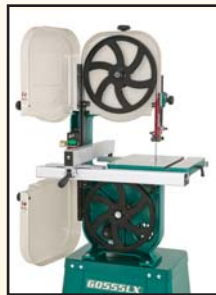
COMPUTER-BALANCED CAST IRON WHEELS WITH RUBBER TIRES
