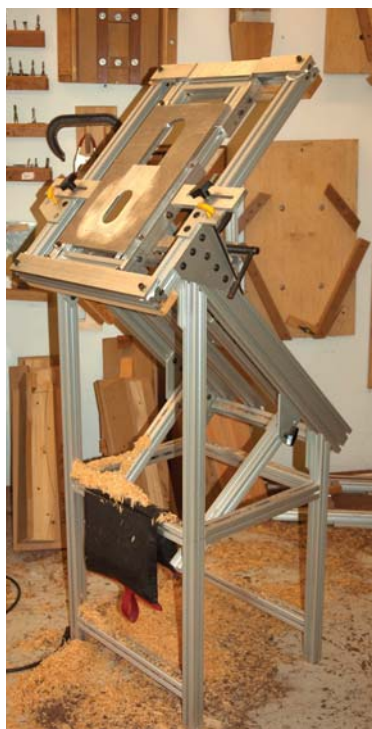
Always a solution. Brian’s “Router Pulpit,” as he calls it, allows him to easily secure and tenon the ends of chair parts of any shape.
