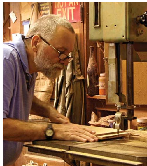
Next step. The large band saw handles a variety of tasks. Here the top and bottom of a tenon is trimmed.
