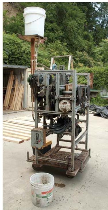
Starting from scratch. Brian’s bark-splitting machine, sometimes referred to as “Hankenstein,” separates layers of bark for weaving chair seats.
