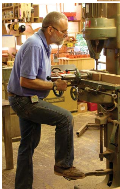
Mortise jig. This pedal-operated hollow-chisel mortiser makes quick work of milling the numerous joints in a Morris chair.
