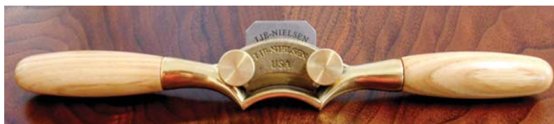
A better spokeshave. Dissatisfied with the surface left from traditional spokeshaves, Brian designed his own (available from Lie-Nielsen Toolworks), which creates a finish-ready surface fresh off the shave.
