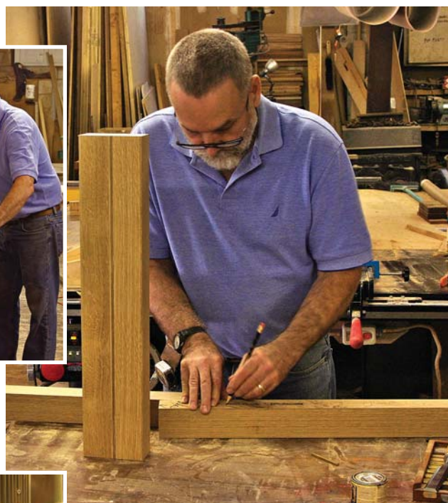
Marking made easy. Dale uses patterns for mortise layout; it's fast, accurate and consistent.
