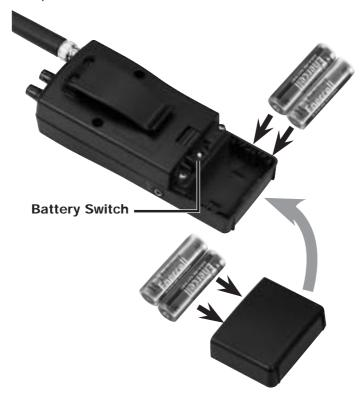
**Warning:** Only set the **Battery Switch** to **Ni-MH** for use with nickel metal hydride (Ni-MH) rechargeable batteries.
