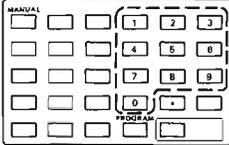
A diagram of the scanner's keypad. The top row has a [MANUAL] button followed by three empty display boxes. The second row has three empty display boxes and buttons 1, 2, and 3. The third row has three empty display boxes and buttons 4, 5, and 6. The fourth row has three empty display boxes and buttons 7, 8, and 9. The fifth row has three empty display boxes, a 0 button, a * button, and a blank button. The sixth row has three empty display boxes, a PROGRAM button, and a blank button. |
