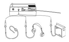
Note: Connecting any external device to the EXT SP jack automatically disconnects the internal speaker.
