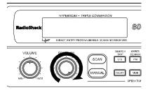
2. Press POWER to turn on your scanner. The scanner continuously scans the unlocked channels.
