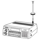
The scanner's sensitivity depends on the antenna's length and various environmental conditions. For the best reception of the transmissions you want to hear, adjust the antenna's length.
