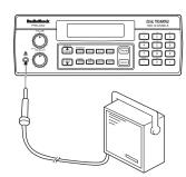
**Note:** Connecting an external speaker disconnects the scanner's internal speaker.
