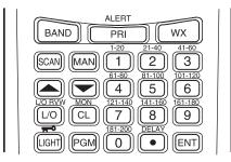
**Note:** Some of the scanner's keys perform more than one function and are marked with more than one label. The steps in this Owner's Manual show only the label on the key appropriate to the action being performed.
