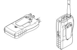
To make your scanner easier to carry when you are on the go, use the supplied belt clip. Use a Phillips screwdriver and the supplied screws to attach the clip to the scanner.
