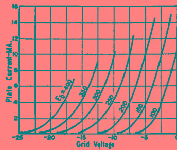
Fig. 3-6 — Grid-voltage-vs.-plate-current curves at various fixed values of plate voltage ( E_b ) for a typical small triode. Characteristic curves of this type can be taken by varying the battery voltages in the circuit at the right.
