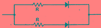
Fig. 5-11 — Diodes in parallel should have equalizing resistors. See text for appropriate value.
