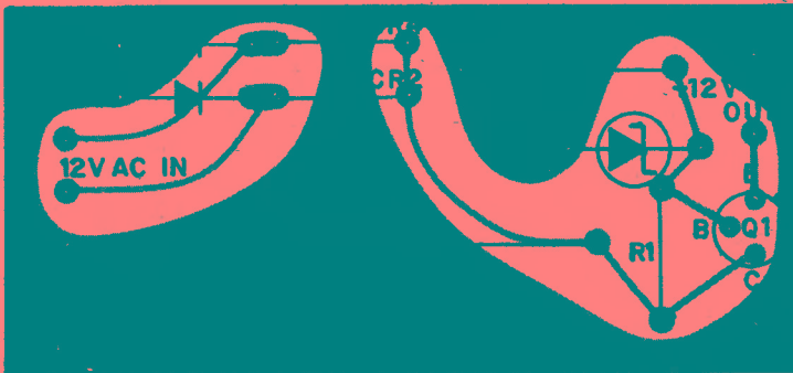
Fig. 7 — Schematic diagram and parts-placement guide for the power supply to the converters. The transformer is mounted external to the board. Pc board size is identical to the one used for the converters.
