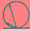
Fig. 21-6 — Illustrating the importance of vertical angle of radiation in determining antenna directional effects. Off the end, the radiation is greater at higher angles. Ground reflection is neglected in this drawing of the free-space pattern of a horizontal antenna.
