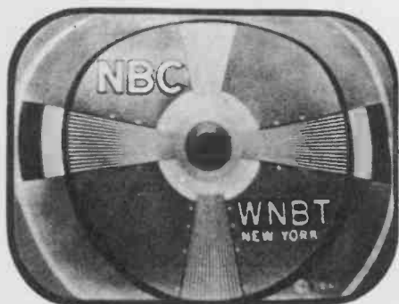
Fig. 9. VERTICAL LINEARITY Misadjusted
