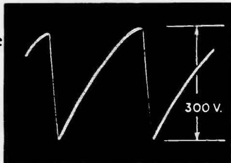
WAVEFORM - OUTPUT OF VERTICAL OSCILLATOR AMPLIFIER TUBE - ONE HALF (PIN #2 OF V-8 AND B-)
