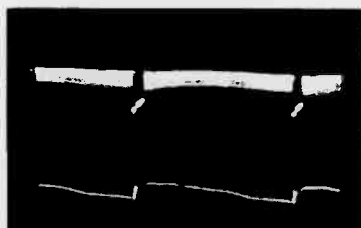
Figure 41—Horizontal (9 Volts PP)
