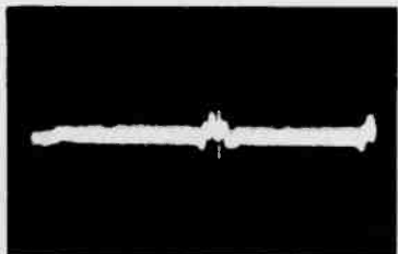
Figure 66—Cathode of Hor. Sync. Discr. (Pin 5 of V123) (6AL5)
