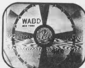
Outside Interference Caused By Diathermy
