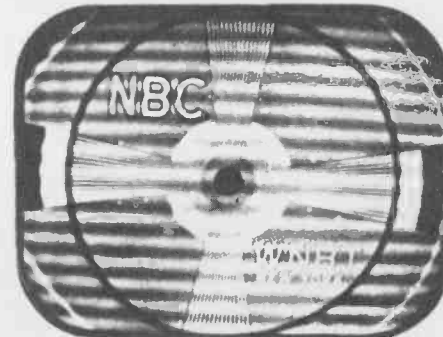
Fig. 6. FINE TUNING Misadjusted
