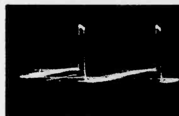
Terminal "E" of Sync Discriminator Transformer (T108)
