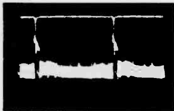
Figure 45—Horizontal (35 Volts PP)
