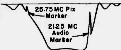
Fig. 31. De-tuned Overall Video IF Response
