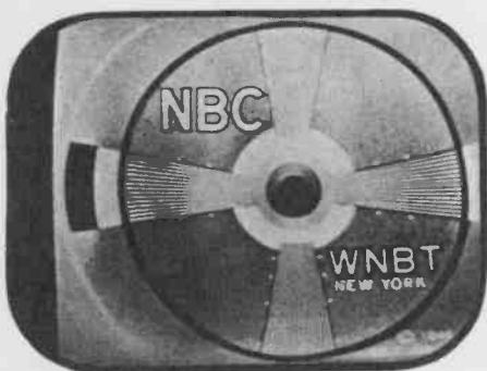
Fig. 8. HORIZONTAL POSITIONING Misadjusted
