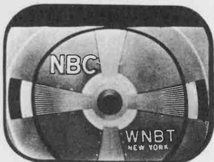
Fig. 7. VERTICAL POSITIONING Misadjusted
