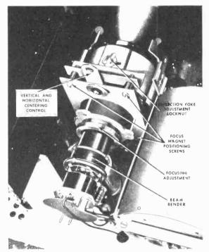
Fig. 29 Mechanical Focus and Centering Adjustments.
