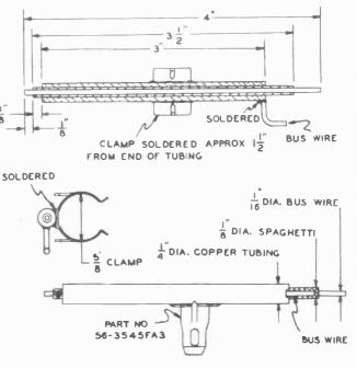
Figure 2. I-F Alignment Jig
