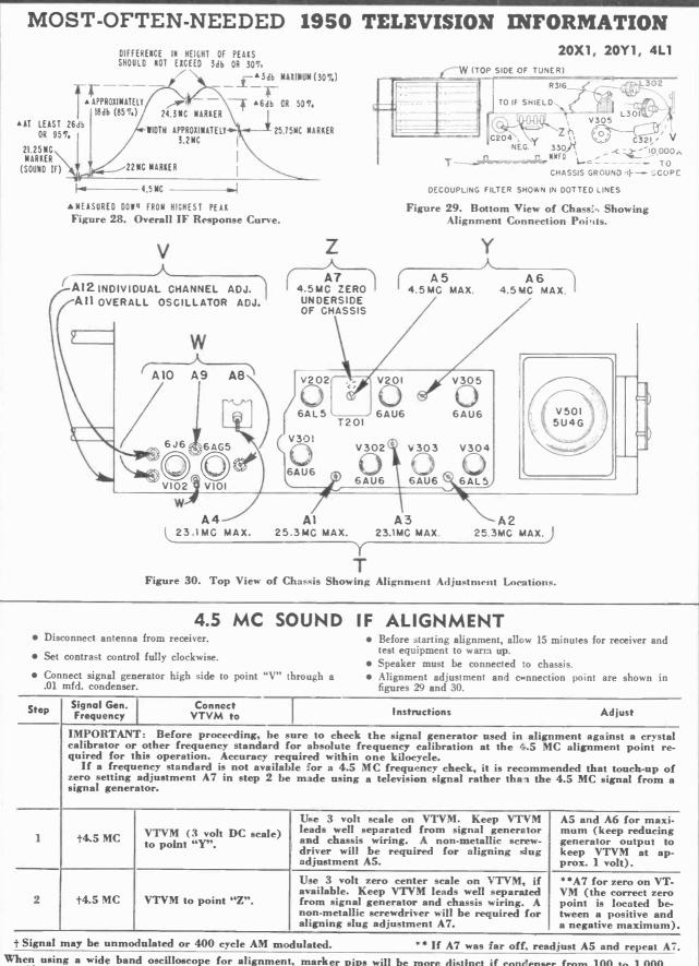
When using a wide band oscilloscope for alignment, marker pips will be more distinct if condenser from 100 to 1,000 mmfd. is connected across the oscilloscope input. Caution: Use the lowest capacity condenser possible, since too high capacity will affect the shape of the response curve.
