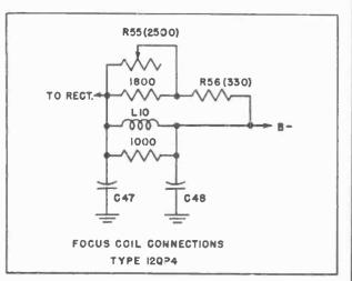
Fig. 5-11 Use of Type 12QP4 Kinescope
