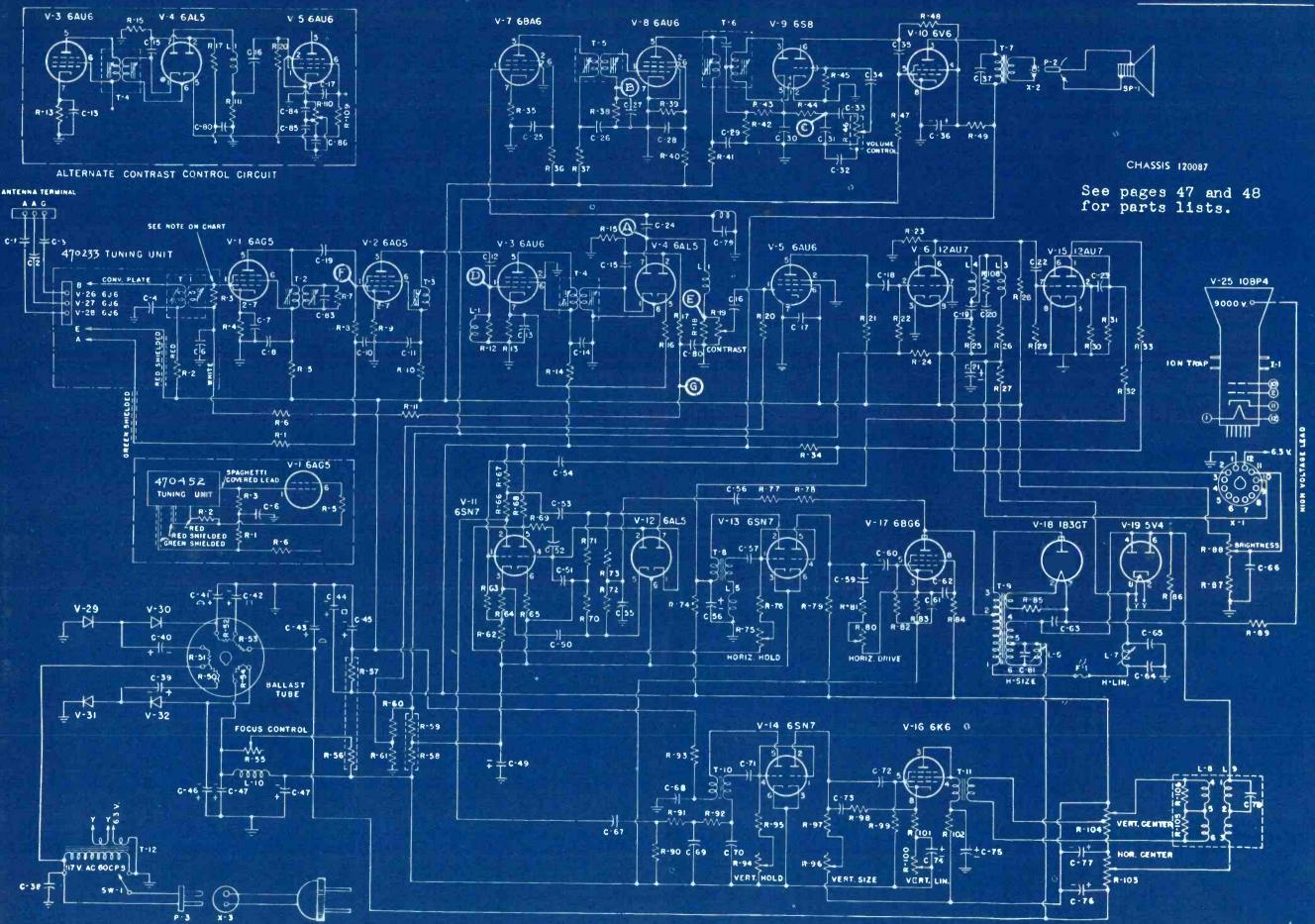
Fig. 5-16 Schematic Diagram-Chassis 120087D
