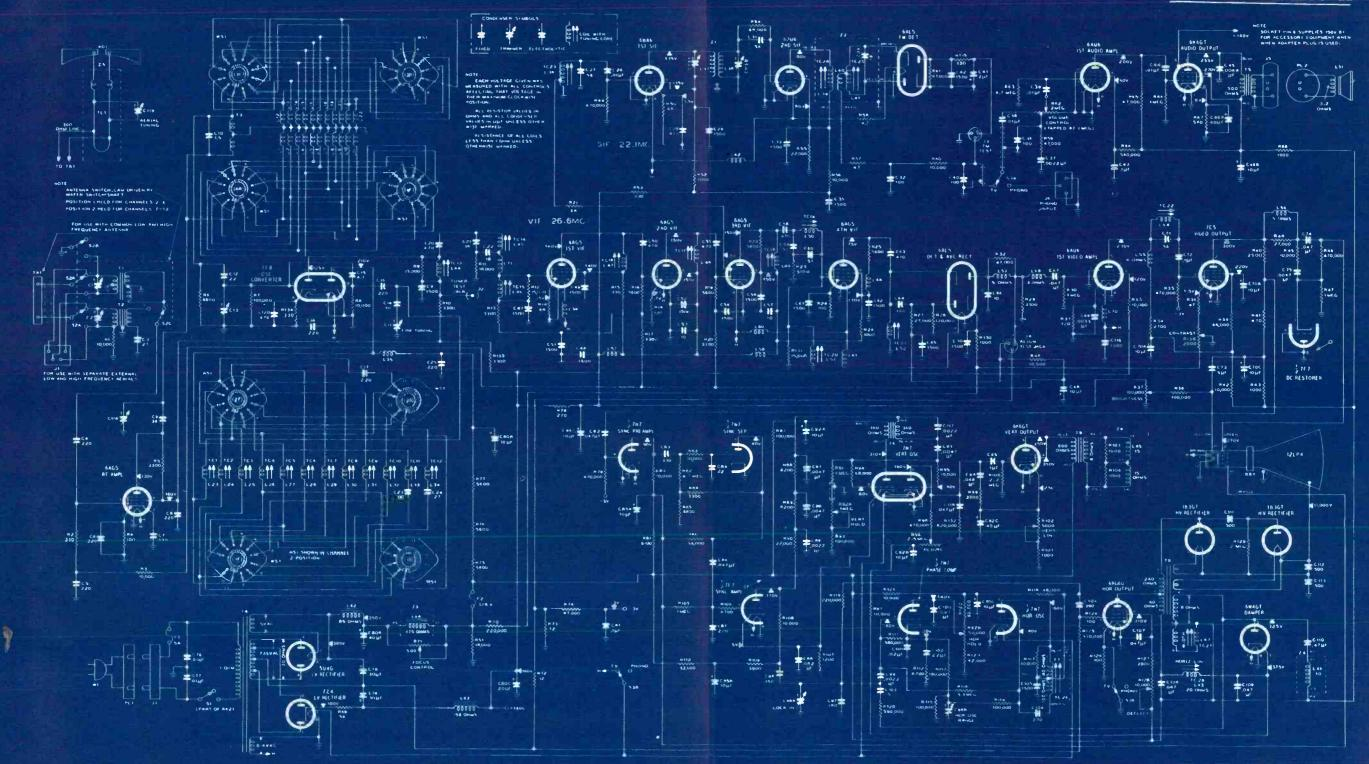
Phileo Television Receiver Model 50-T1443, Code 122, Complete Schematic Diagram
