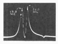
Figure 31—Response of Third Pix I·F Transformer
