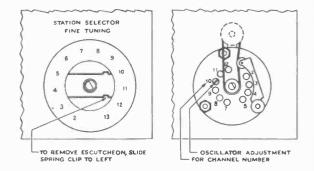
Figure 7-R-F Oscillator Adjustments
