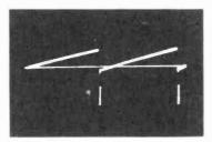
Figure 64—Grid of Vertical Output (140 Volts PP) (Pin 5 of V111) (6K6GT) -----
