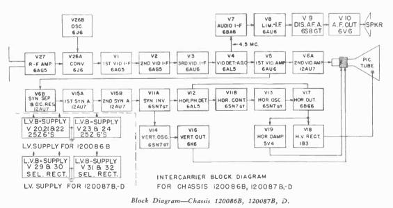
(Note-Chassis 120066 differs from the above in that the audio i-f is 21.25 mc. and is taken from V-1; the low voltage supply is similar to Chassis 120086B, but does not use a ballast tube; Chassis 120066B does use a ballast tube.)
