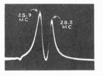
Figure 30—Response of Second Pix I-F Transformer
