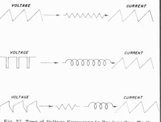
Fig. 22 Type of Voltage Necessary to Produce Saw-Tooth Current Through a Resistance, Inductance and the Combination of Resistance and Inductance.
