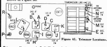
Trimmer adjustments A, C, G, H, J, made from underside of chassis.
