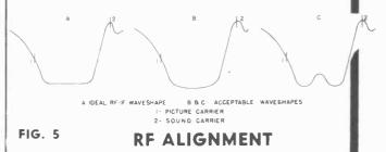
In the alignment of the RF section of this receiver three pieces of test equipment are necessary: a sweep generator, a signal generator and a cathode Ray Oscilloscope.
