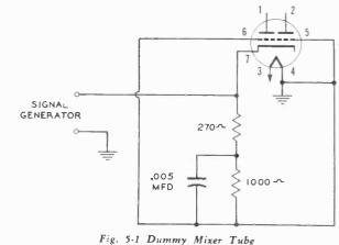
NOTE—Carefully bend Pin 7 at right angle, connect Pin 5 and 6 to Pin 4 which is grounded at the socket. Connect other components as shown.
