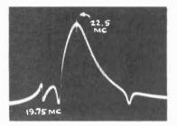
Figure 33—Response of Fifth Pix I-F Transformer
