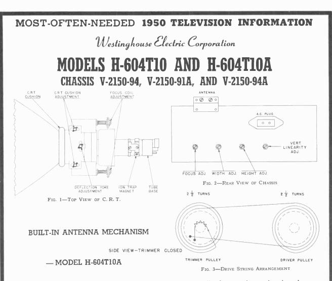
The antenna trimmer control is designed to rotate through a range of 21/2 turns. At one extreme of rotation the trimmer is completely closed, thus serving as a stop. A collar locked on the threaded portion of the trimmer shaft serves as a stop at the other extreme of rotation. When the trimmer shaft is rotated 21/2 turns from the completely closed position, the collar on the shaft should bear against the metal shoulder on the trimmer and stop rotation in that direction.
