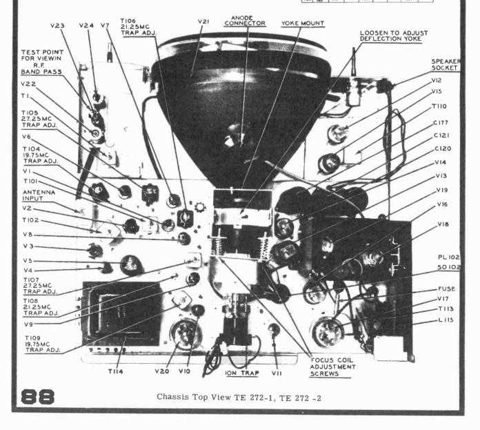
OSCILLATOR TOUCH-UP. All channels should come in best with the same approximate setting of the Fine Tuning Control.
