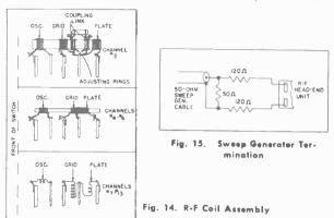
nated as shown in Figure 15. The resistors used should be noninductive. The marker signal generator may be loosely coupled through a small capacitor to the same point of input as the sweep generator
