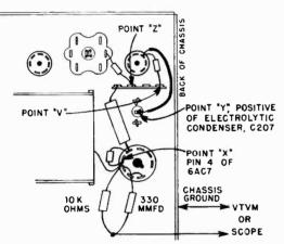
Figure 29. Alignment Connection Points.
