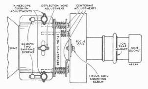
Figure 3-Yoke and Focus Coil Adjustments
