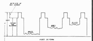
Fig. 19 Composite Video Signal.
