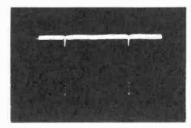
Output of 1st Sync Separator (Pin 2 of V109) (6SN7GT)
