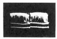
Output of 2nd Video Amplifier (Pin 3 of V107) (6K6GT) (Picture Max.)
