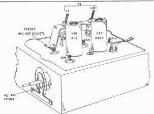
Fig. 5-9 Alignment Points-Tuner 470452
