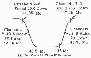
Inject a 47.25 marker and adjust trap L60 for minimum indication on the scope or on a VTVM connected to the video detector.
