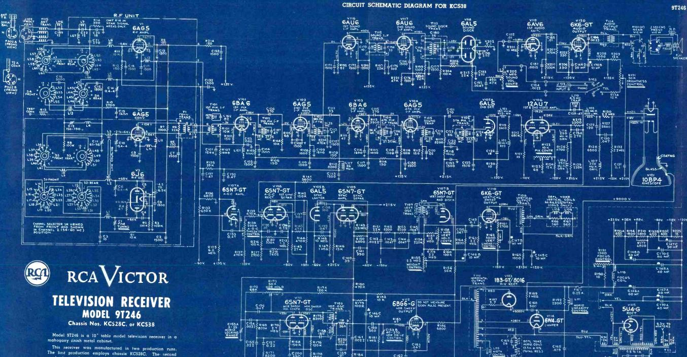
This receiver was manufactured in two production runs. The first production employs chassis KCS28C. The second production employs chassis KCS38, which is similar to KCS28C. However, KCS38 represents a change of tube types in three sockets, it employs a different speaker, focus coil power transformer, horizontal and vertical output transformers, picture i-f transformers as well as circuit changes.
