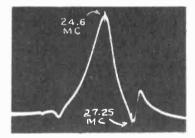
Figure 32-Response of Fourth Pix I-F Transformer
