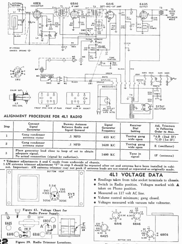
Figure 40. Voltage Chart for 4L1 Radio.
